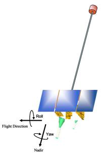
The spacecraft will be permanently nadir pointing. Relaxed communication antenna pointing requirements do not require the micro-satellite to maneuver. A simple design incorporating a gravity-gradient boom controls pitch and roll axes. A momentum bias wheel and magneto-torquers provide yaw axis control and initial attitude capture.
