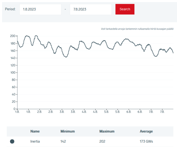
Figure 4: Instantaneous reserve in the Nordic Power System (Europe) - first week of August 2023 [8]
