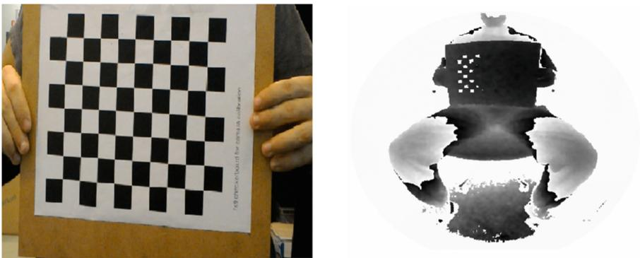
**Fig. 3.** A quasi-synchronized shot from the RGB camera (left) and the short-range depth camera (right).
