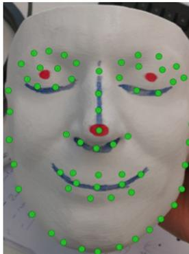
**Fig. 6.** The Dlib face detection software locating the face landmarks on a 3D-printed head [6].
