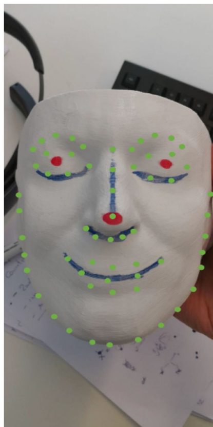
Fig. 6 Facial landmarks (in green) detected over a phantom head. The red dots are used to measure the registration error and not related to this stage. (For interpretation of the references to color in this figure legend, the reader is referred to the web version of the article)
