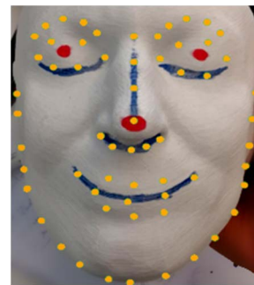
Figure 3 – Pattern recognition algorithm applied on a picture of the printed 3D model. In orange the landmark points.
