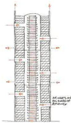
Figure 7: Building section of the model building
