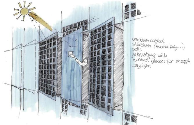
Vacuum coated silicium cells (monocrystalline, polycrystalline) could be alternating with the normal 12mm glasses in order to still get enough daylight into the offices. These cells could produce energy to cover the amount of energy for lightning etc... The surplus energy could be supplied into the local energy network.
