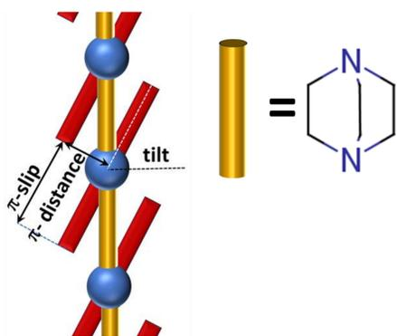
**Solution: maximize hole transport by using DABCO as apical linker**
