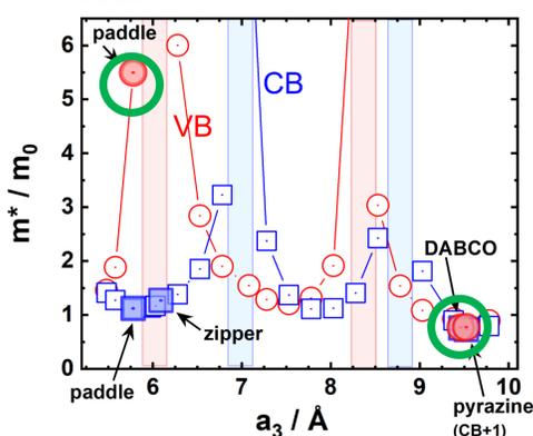
Effective mass as a function of the stacking distance between Zn paddlewheels
