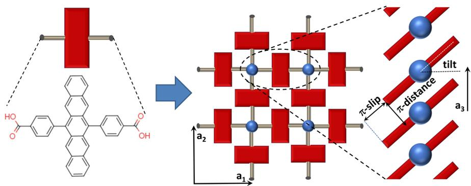
Schematic structure of the idealized orthorhombic pentacene MOF [3]
