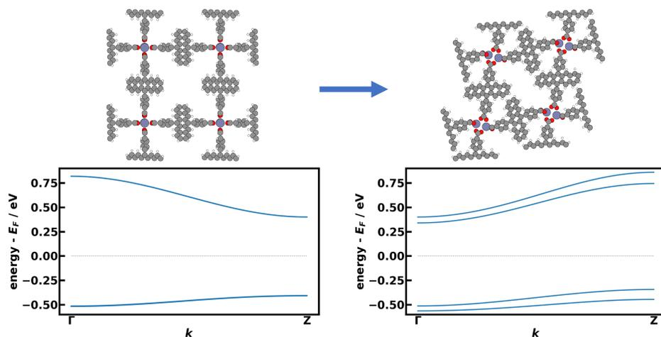
PBE-calculated frontier bands for the idealized orthorhombic structure (left) and the fully relaxed triclinic structure (right)
