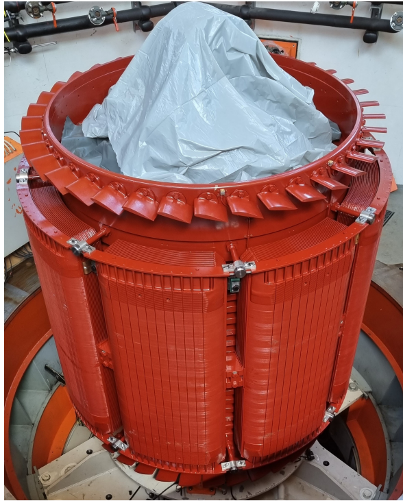
Figure 25: Rotor of a vertical salient-pole synchronous machine
