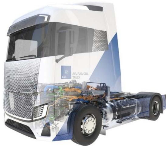
Figure 7-1: AVL HD Fuel Cell Technology Demonstrator Truck [34]
