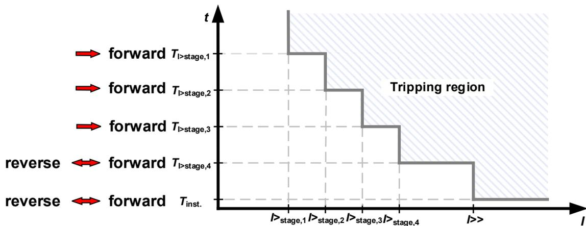
Figure 2: Example of a multi-stage DTO tripping characteristic with directional dependence and high-current stage (based on [2], page 126, Figure 4.7)
