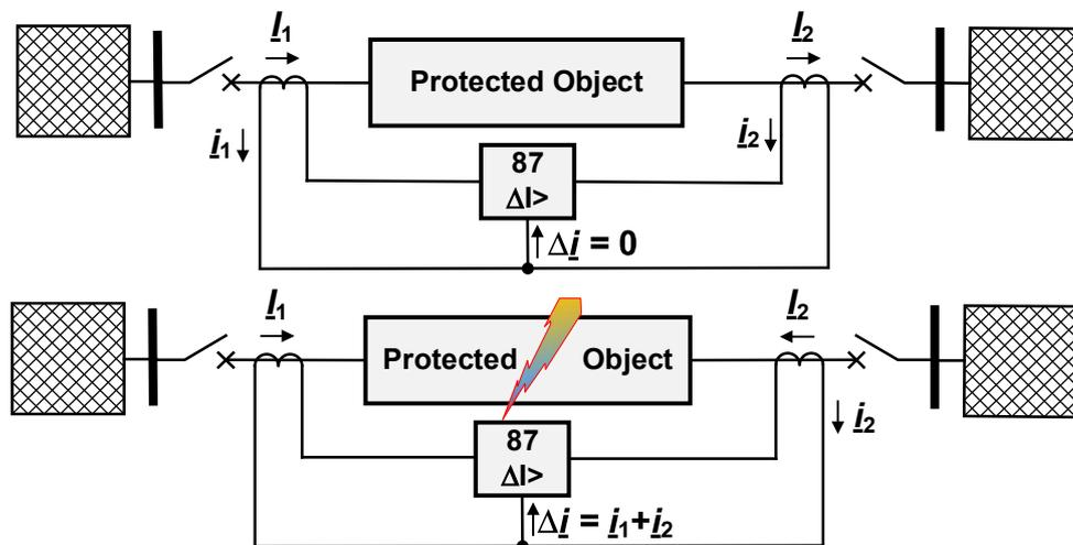
Figure 12: Basic topology for differential protection; above: normal operation; below: fault
