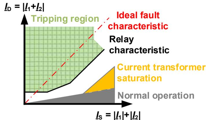
Figure 13: Relay characteristic of a differential protection device
