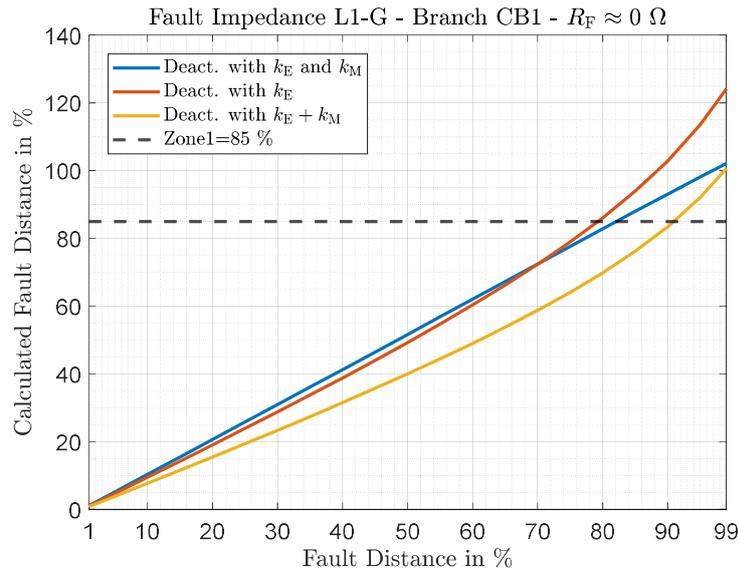
Figure 71: Rel. calculated fault distance for L-G fault for monitoring mode of the SSSC and  $R_f \approx 0 \Omega$ ; analysis of the impact of  $k_M$
