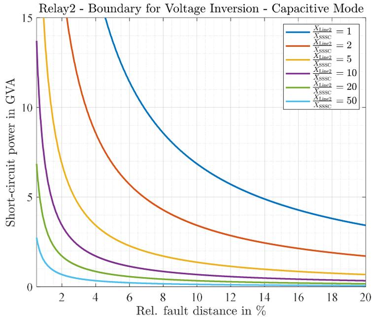
Figure 61: Voltage inversion boundary for multiple values of  $X_{Line2}/X_{SSSC}$
