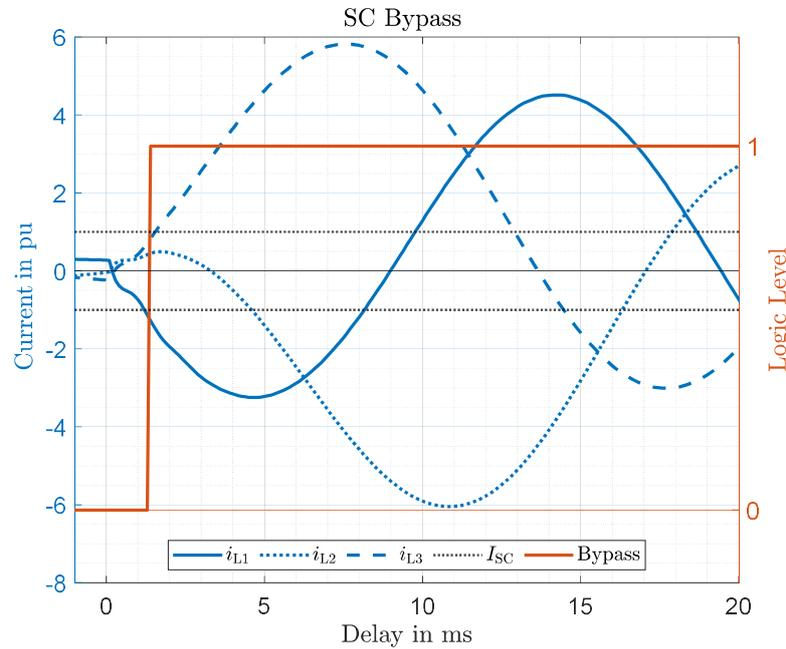
Figure 35: Instantaneous current protection for a three-phase short-circuit
