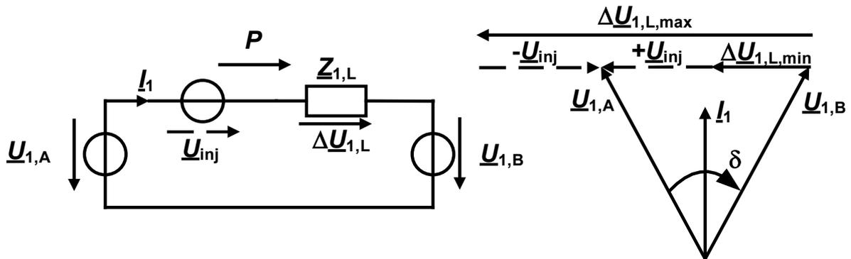
Figure 20: Phasor diagram for capacitive and inductive operation of a SSSC based on [9]
