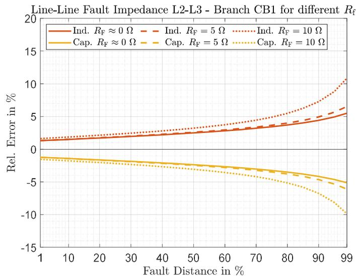
Figure 66: Relative measurement error in branch CB1 for L-L fault, for inductive and capacitive operation of the SSSC and different  $R_f$
