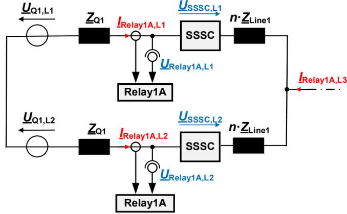
Figure 38: Equivalent circuit L1-L2 of a three-phase fault (L1-L2-L3), based on Figure 37 while neglecting the fault resistance  $R_f$
