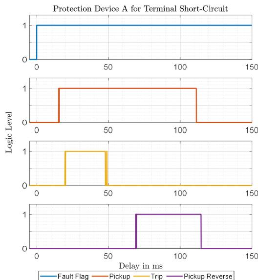
Figure 91: Pickup, pickup reverse and trip signals for P433 for memorised voltage threshold  $U_{th} = 4\%$
