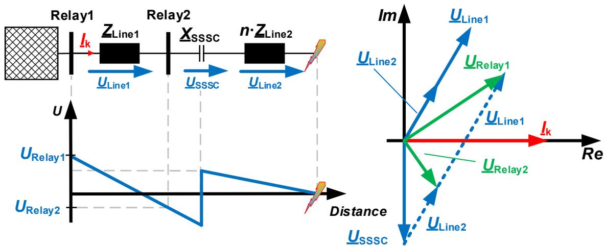
Figure 22: Voltage inversion based on [3,5]
