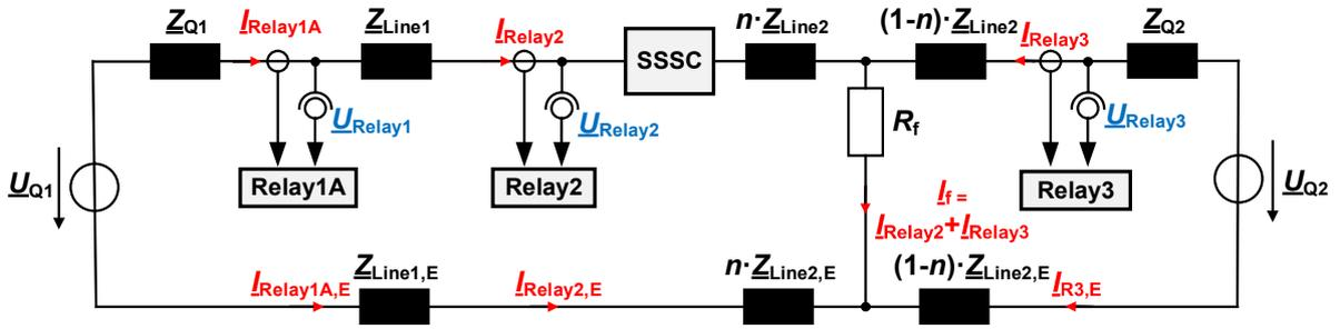
Figure 47: Equivalent circuit L-G of a one-phase fault (L-G), based on von Figure 45 while considering the fault resistance  $R_f$  and double infeed
