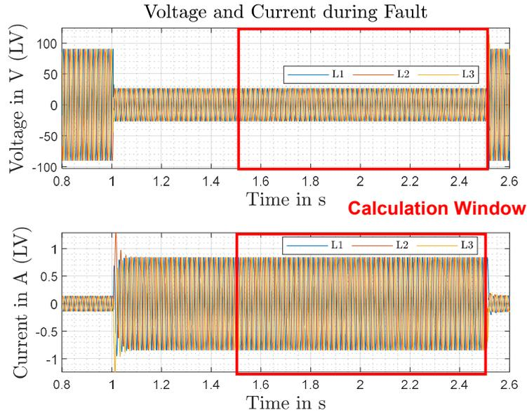
Figure 64: Steady-state short circuit window for impedance calculation
