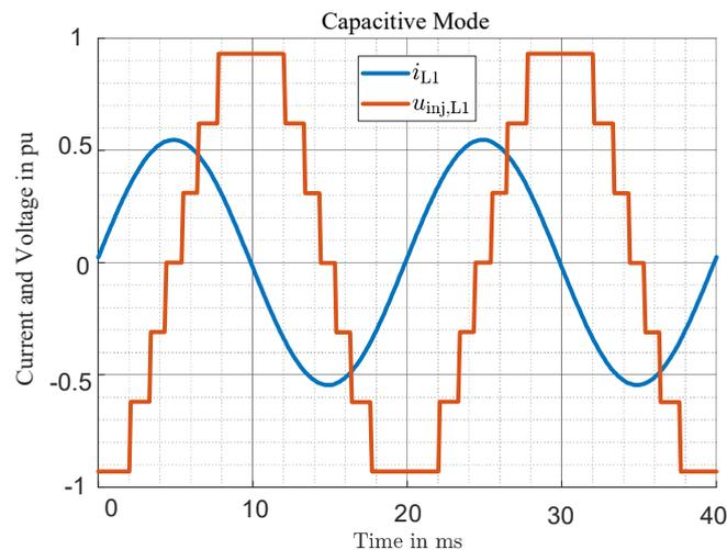
Figure 31: SSSC operating capacitive
