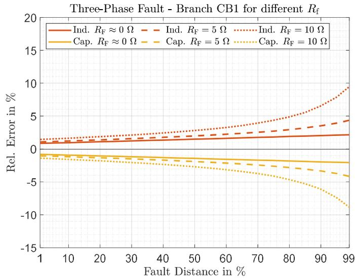
Figure 67: Relative measurement error in branch CB1 for three-phase fault, for inductive and capacitive operation of the SSSC and different  $R_f$
