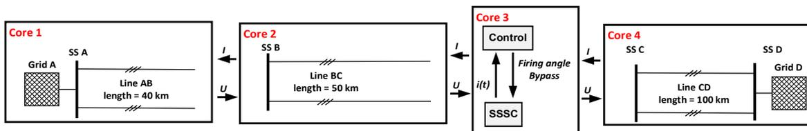
Figure 78: Multicore application with the Simulink model separated on all four cores
