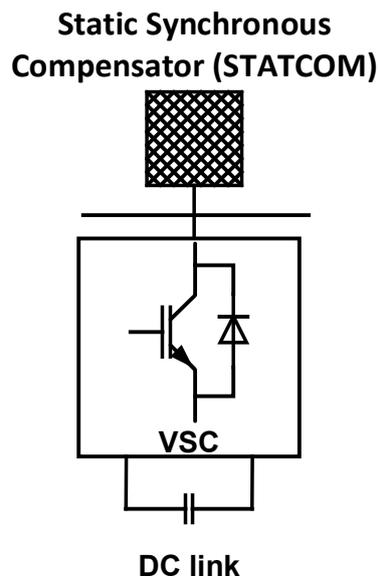
Figure 15: Static Synchronous Compensator (STATCOM) based on [9]
