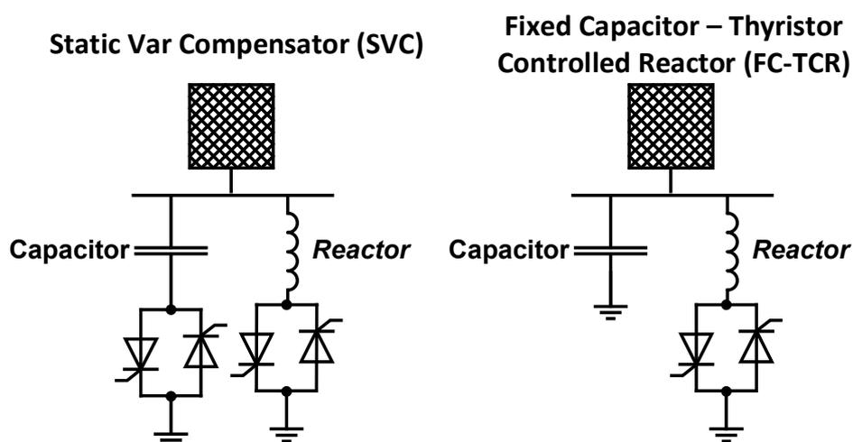
Figure 14: Static Var Compensator SVC and Fixed Capacitor - Thyristor Controlled Reactor FC-TCR, based on [9]
