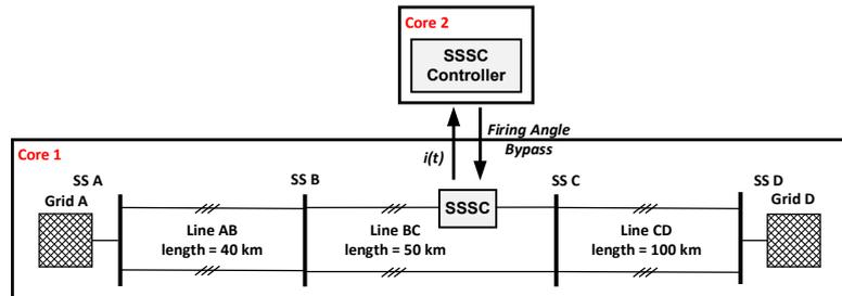
Figure 79: Final solution for real-time simulation
