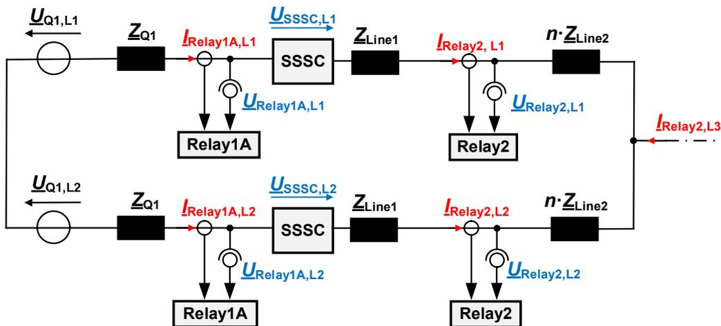
Figure 50: Equivalent circuit L1-L2 of a three-phase fault (L1-L2-L3), based on Figure 49 while neglecting the fault resistance  $R_f$
