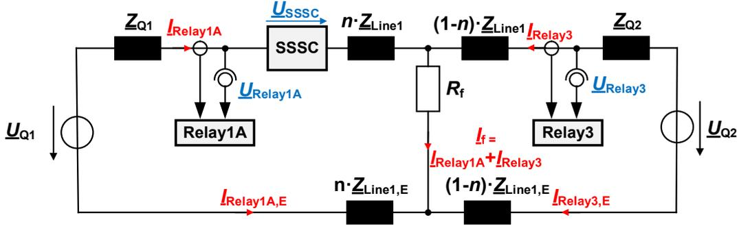
Figure 39: Equivalent circuit L-G of a one-phase fault (L-G), based on Figure 37 while considering the fault resistance  $R_f$  and double infeed
