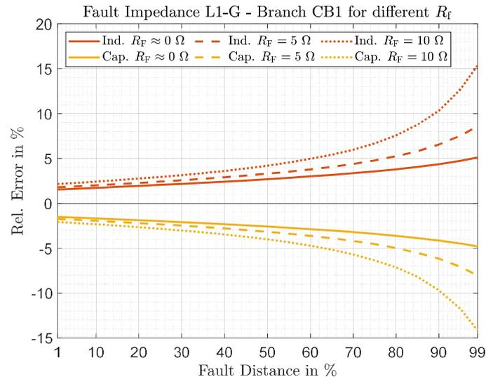
Figure 65: Relative measurement error in branch CB1 for L-G fault, for the inductive and capacitive operation of the SSSC and different  $R_f$
