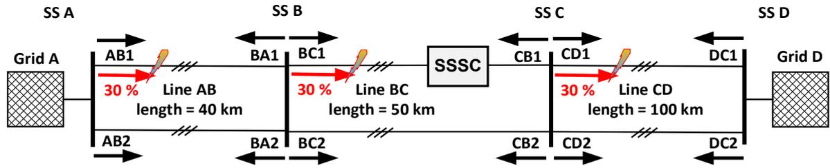
Figure 63: Grid topology for one-, two- and three-phase short-circuit calculations with the SSSC operating inductive, capacitive or being deactivated and the fault location 30% of line length
