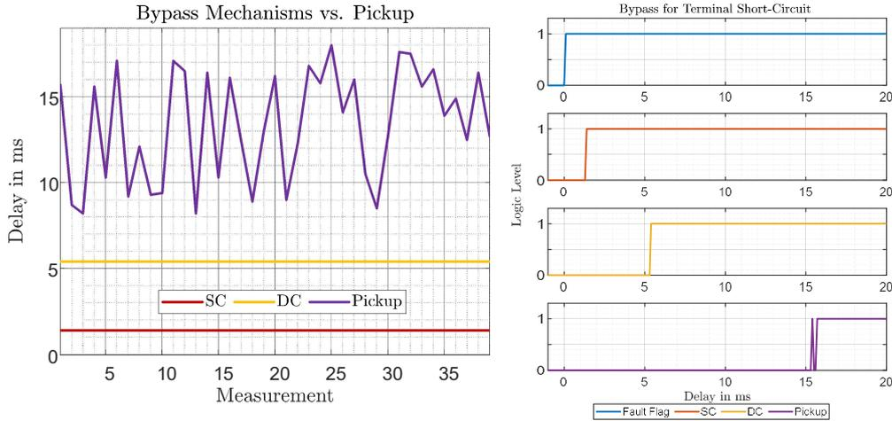
Figure 92: Automatic bypass speed vs. pickup speed of P433
