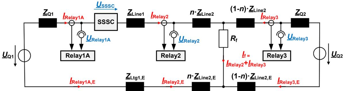
Figure 51: Equivalent circuit L-G of a one-phase fault (L-G), based on von Figure 49 while considering the fault resistance  $R_f$  and double infeed
