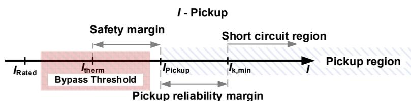
Figure 80: Coordination of the instantaneous current threshold of the SSSC with the overcurrent pickup of distance protection based on Figure 4
