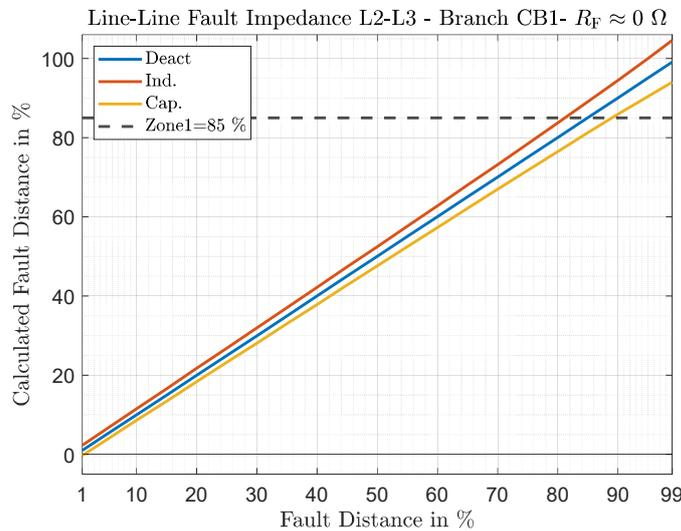
Figure 68: Rel. calculated fault distance for L-L fault for inductive and capacitive operation of the SSSC and  $R_f \approx 0 \Omega$
