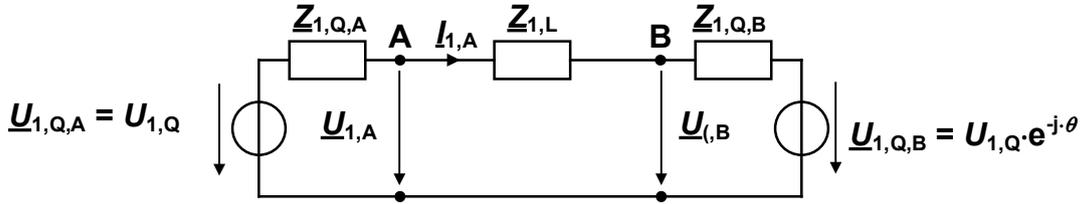
Figure 10: Simplified equivalent circuit for explaining power swings based on [4]
