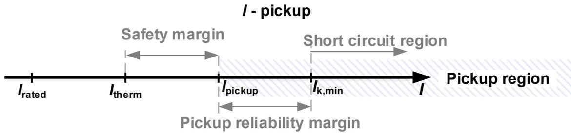
Figure 4: Overcurrent pickup for distance protection based on [4]
