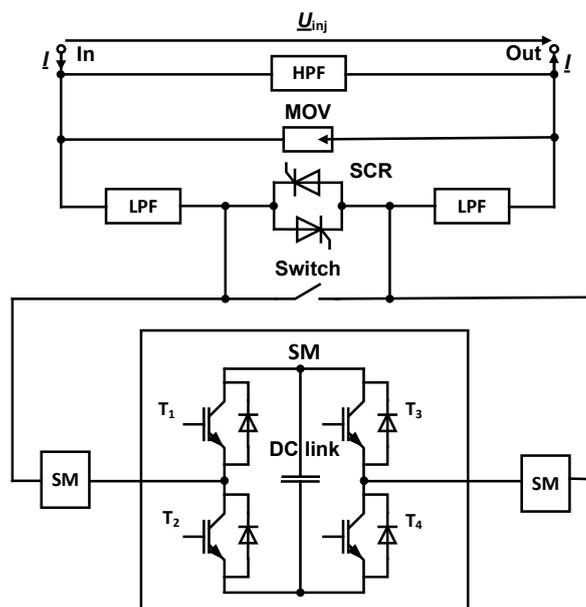
Figure 18: Modular Static Synchronous Series Compensator (m-SSSC) [11]
