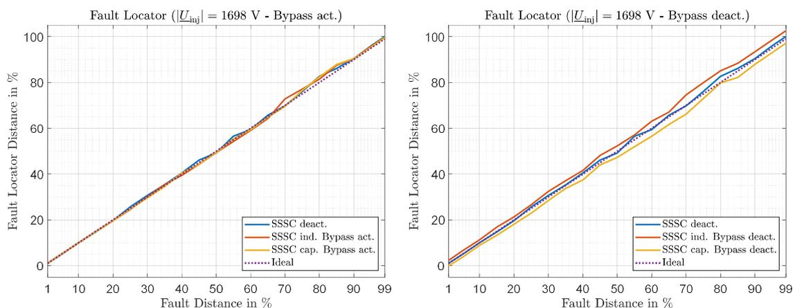
Figure 81: Measured fault distance by the fault locator of protection device P433 for the bypass of the SSSC being activated and deactivated (bypass failure) for  $|\underline{U}_{inj}| = 1698 \text{ V}$
