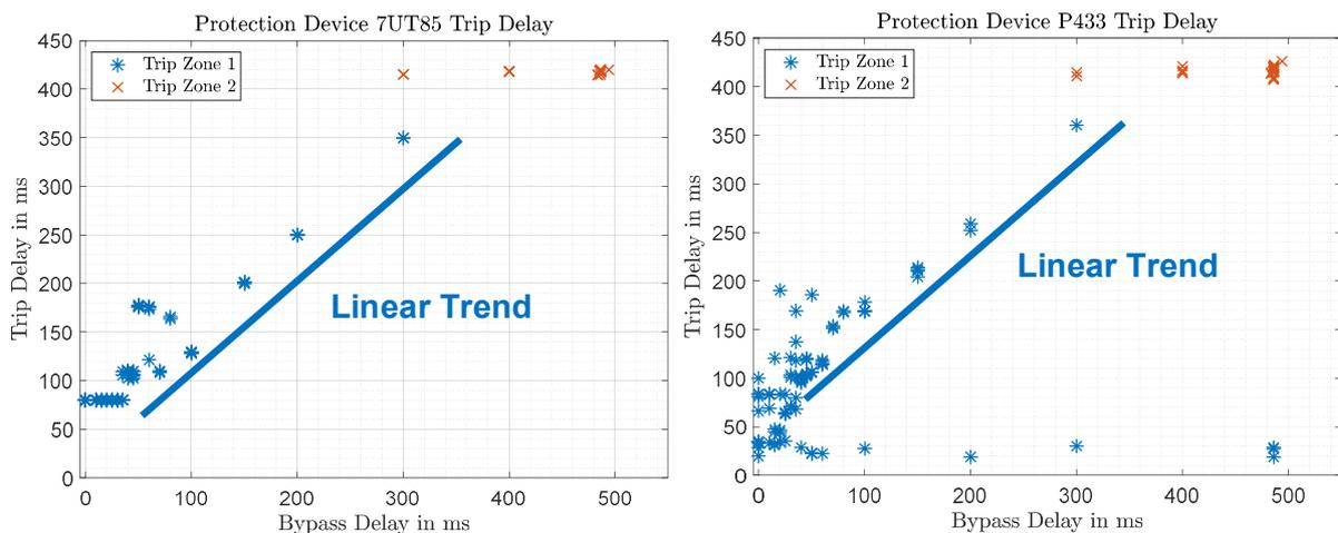
Figure 86: Zone shift from Z1 to Z2 (underreach) in dependency of bypass delay for 7UT85 (left) and for P433 (right)
