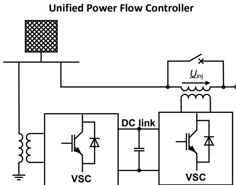
Figure 21: Unified Power Flow Controller (UPFC) based on [9]
