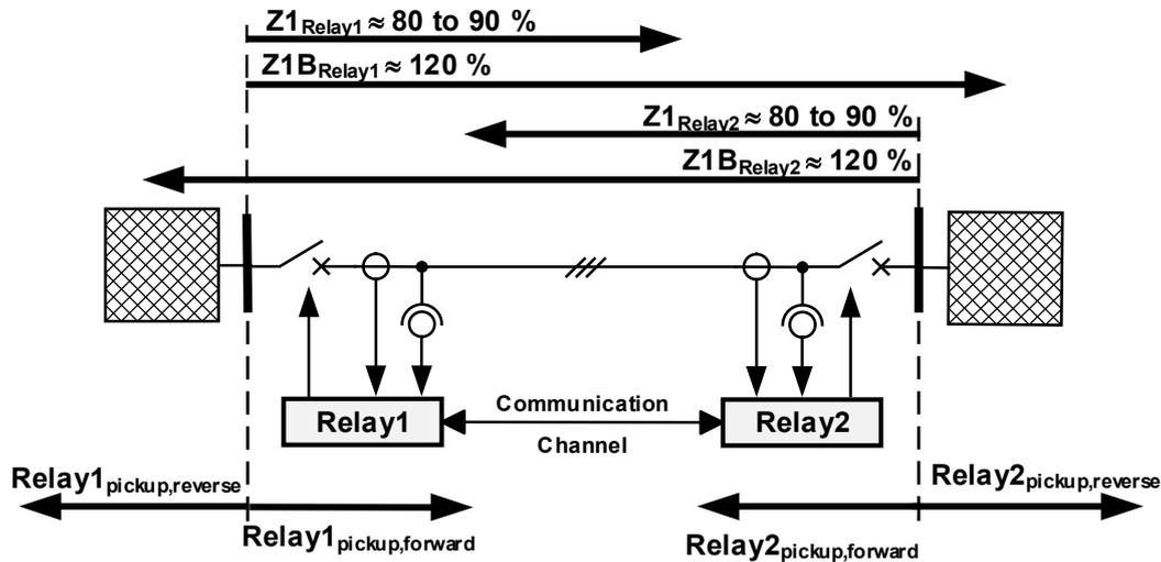
Figure 9: Teleprotection setup with two relays Relay1 and Relay2
