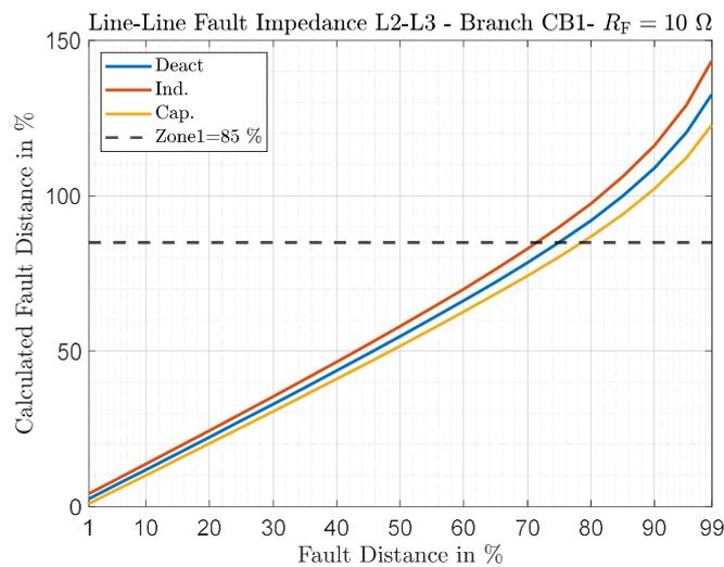
Figure 70: Rel. calculated fault distance for L-L fault for inductive and capacitive operation of the SSSC and  $R_f = 10 \Omega$
