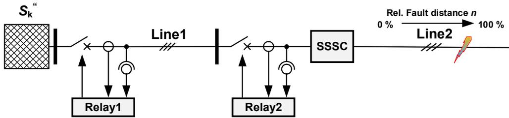
Figure 53: Grid topology for the assessment of the impact of the SSSC on the relay's grading and the occurrence of voltage- and current inversion
