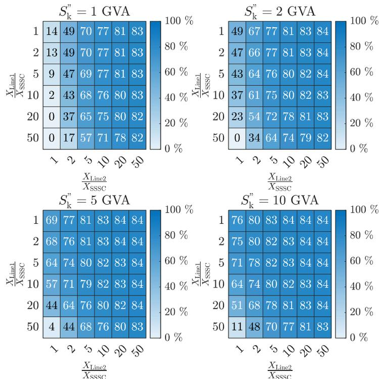
Figure 54: Zone shifting Z1 to Z2 for Relay 2 for inductive operation mode of SSSC; ideal = 85 %
