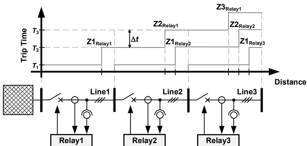
Figure 8: Grading plan of three distance protection devices Relay1, Relay2 and Relay3
