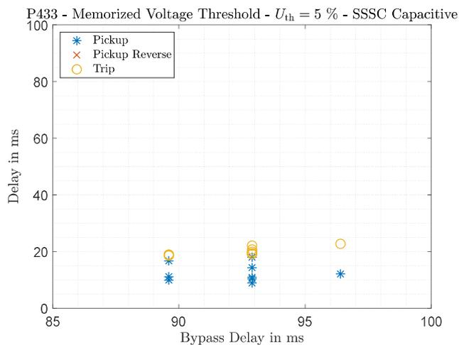
Figure 89: Pickup and trip signals for P433 for memorised voltage threshold  $U_{th} = 5\%$
