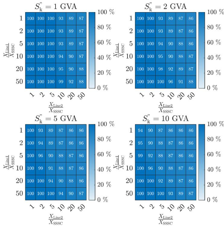
Figure 56: Zone shifting Z2 to Z1 for Relay2 for capacitive operation mode of SSSC; ideal = 85 %
