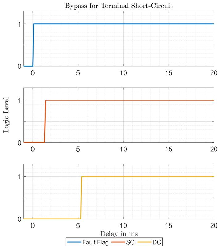
Figure 34: Response of the bypass to a three-phase short-circuit
