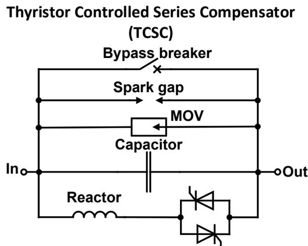
Figure 16: Thyristor Controlled Series Compensator (TCSC) based on [10]
