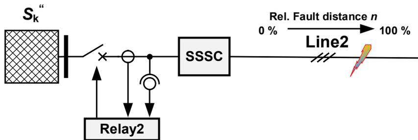
Figure 60: Topology for investigation the voltage inversion boundary for multiple values of  $X_{Line2}/X_{SSSC}$
