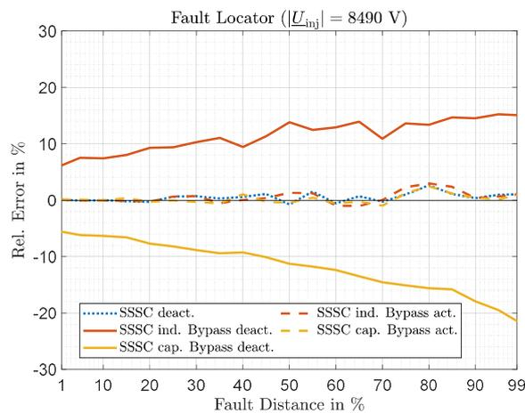
Figure 84: Relative error by fault locator for SSSC deactivated, inductive and capacitive and for bypass activated and deactivated for  $|\underline{U}_{inj}| = 8490$  V
