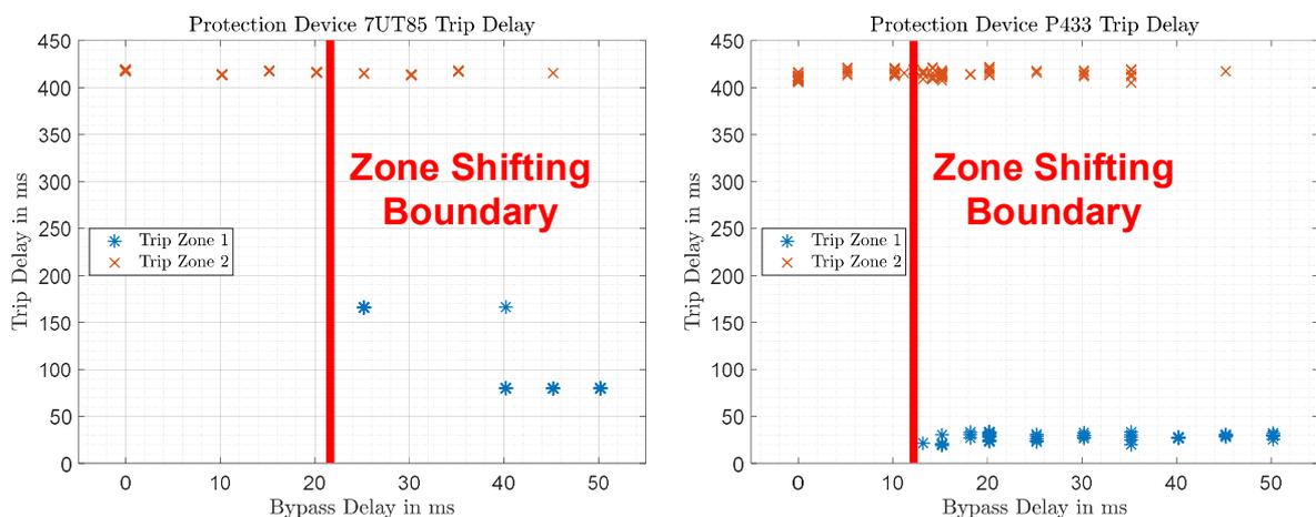
Figure 85: Zone shift from Z2 to Z1(overreach) in dependency of the bypass delay for 7UT85 (left) and P433 (right)
