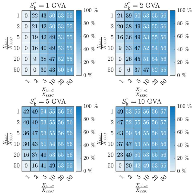
Figure 55: Zone shifting Z2 to Z3 for Relay1 for inductive operation mode of SSSC; ideal = 57 %
