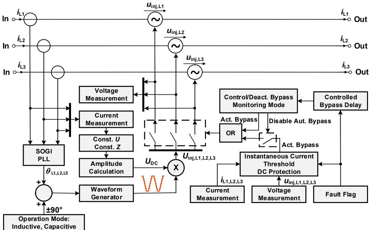
Figure 29: Topology of the SSSC model
