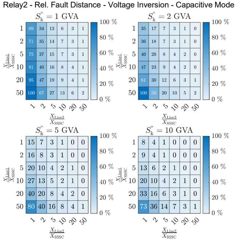
Figure 59: Voltage inversion for Relay 2 for capacitive operation mode of SSSC; ideal = 0 %
