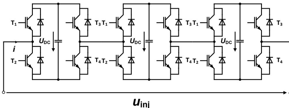
Figure 24: Three SMs for one leg of the SSSC (one phase)
