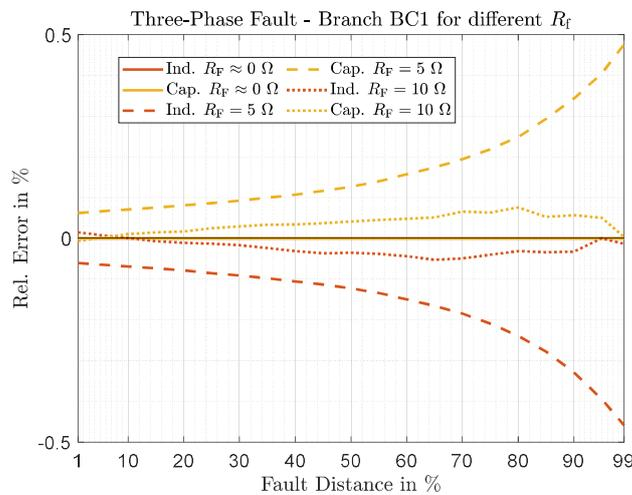
Figure 74: Relative measurement error in branch BC1 for three-phase fault, for inductive and capacitive operation of the SSSC and different  $R_f$
