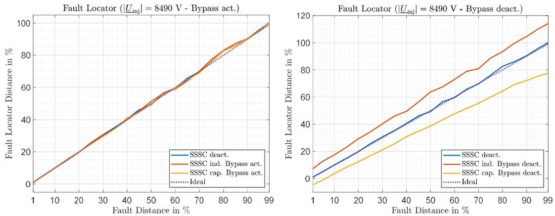
Figure 83: Measured fault distance by the fault locator of protection device P433 for the bypass of the SSSC being activated and deactivated (bypass failure) for  $|\underline{U}_{inj}| = 8490$  V
