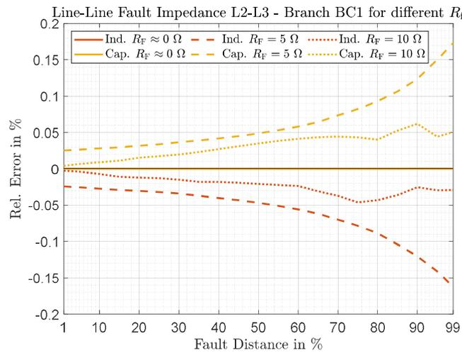
Figure 73: Relative measurement error in branch BC1 for L-L fault, for inductive and capacitive operation of the SSSC and different  $R_f$
