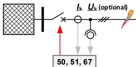
Figure 1: Integration of overcurrent protection
