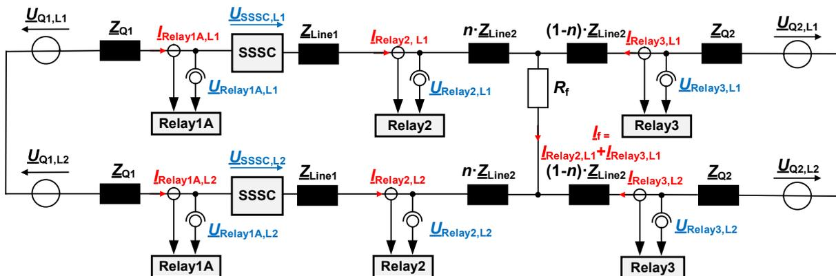
Figure 52: Equivalent circuit L1-L2 of a two-phase fault (L-L), based on Figure 49 while considering the fault resistance  $R_f$  and double infeed
