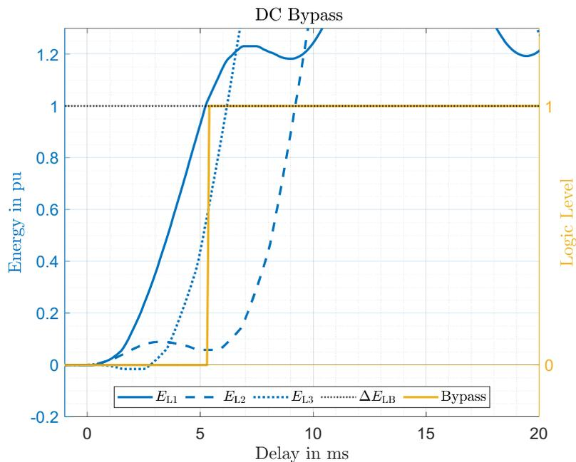
Figure 36: DC protection for a three-phase short-circuit
