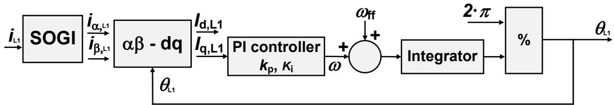
Figure 27: Flowchart for obtaining the reference angle  $\theta_{L1}$
