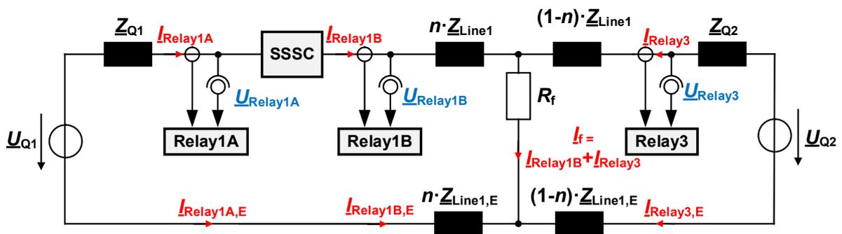
Figure 43: Equivalent circuit L-G of a one-phase fault (L-G), based on Figure 41 while considering the fault resistance  $R_f$  and double infeed
