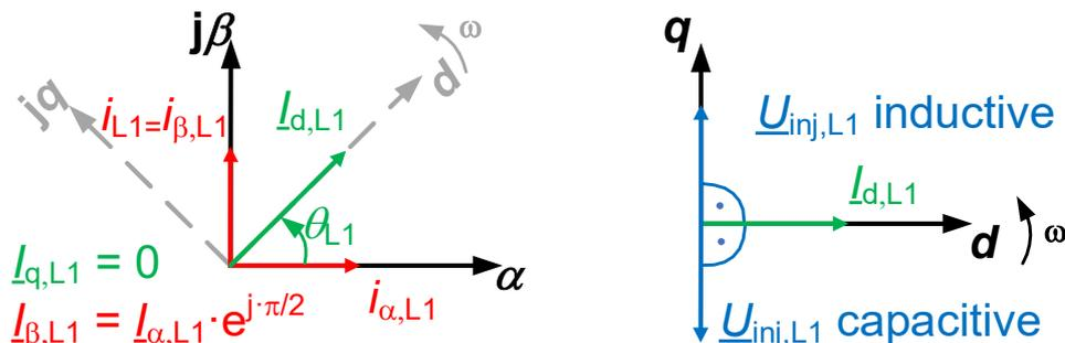
Figure 28: Phasor diagram for SOGI, PLL and rotating reference frame
