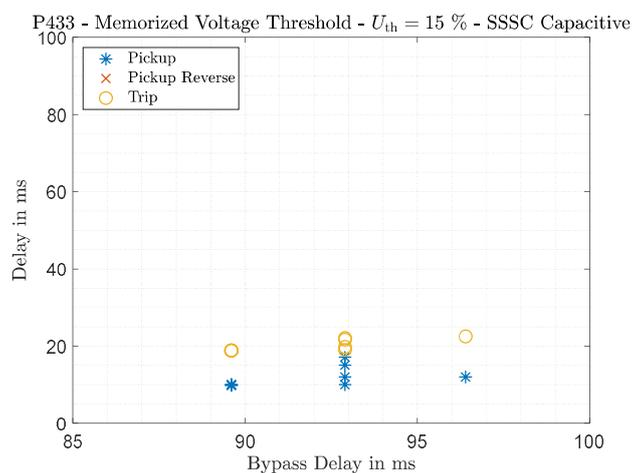
Figure 87: Pickup and trip signals for P433 for memorised voltage threshold  $U_{th} = 15 \%$
