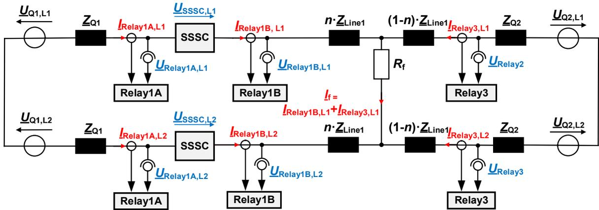
Figure 44: Equivalent circuit L1-L2 of a two-phase fault (L-L), based on Figure 41 while considering the fault resistance  $R_f$  and double infeed
