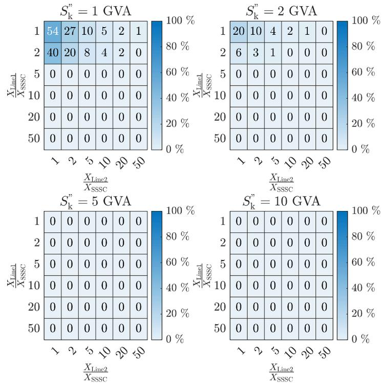
Figure 58: Zone shifting Z2 to Z1 for Relay1 for capacitive operation mode of SSSC; ideal = 0 %
