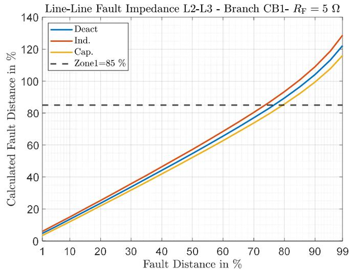
Figure 69: Rel. calculated fault distance for L-L fault for inductive and capacitive operation of the SSSC and  $R_f = 5 \Omega$
