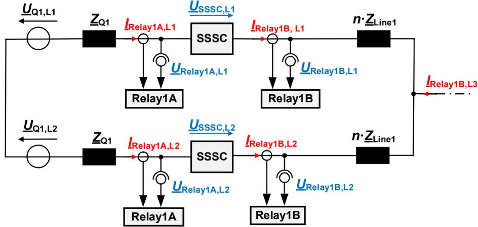
Figure 42: Equivalent circuit L1-L2 of a three-phase fault (L1-L2-L3), based on Figure 41 while neglecting the fault resistance  $R_f$
