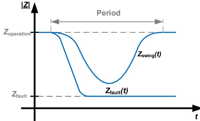
Figure 11: Quantitative progression of absolute impedance values during power swing and fault based on [2]
