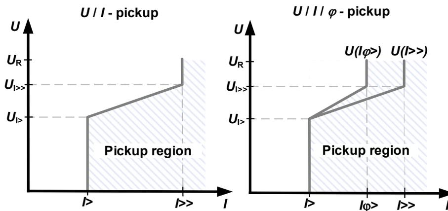
Figure 5:  $U/I$  – pickup (left) and  $U/I/\varphi$  – pickup (right) based on [4]
