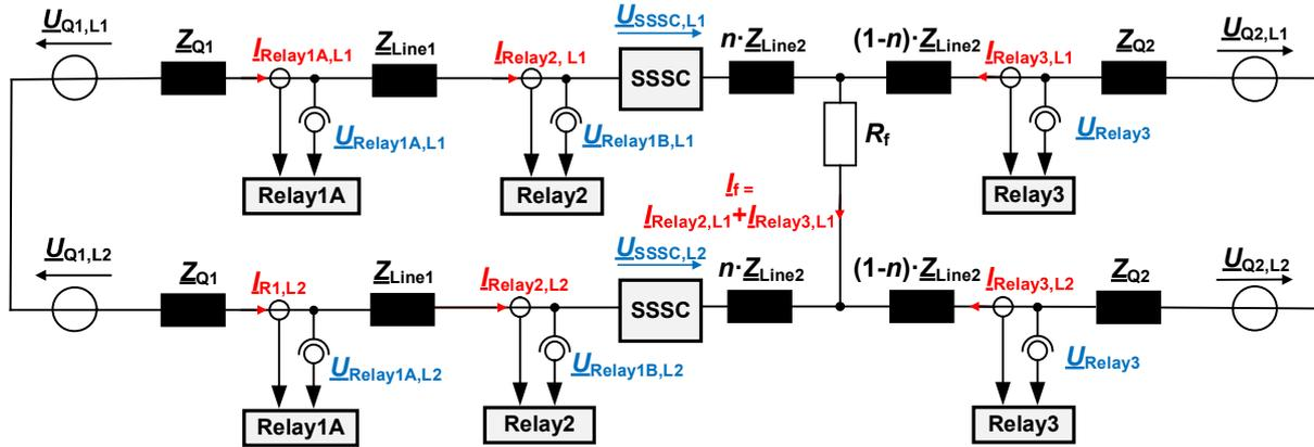
Figure 48: Equivalent circuit L1-L2 of a two-phase fault (L-L), based on Figure 45 while considering the fault resistance  $R_f$  and double infeed
