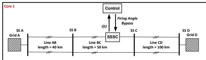
Figure 77: Grid and SSSC implemented on one CPU core
