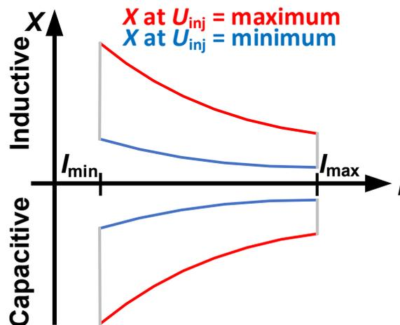
Figure 19: Operational diagram for a SSSC
