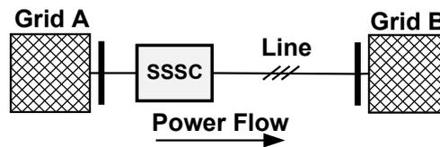
Figure 32: Topology for lossless power flow simulation and calculation
