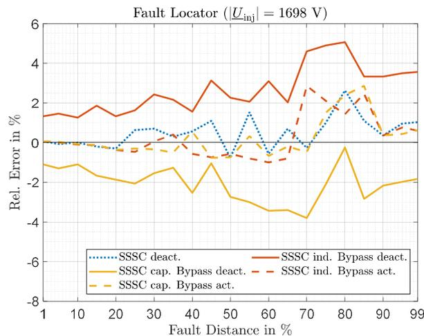
Figure 82: Relative error by fault locator for SSSC deactivated, inductive and capacitive and for bypass activated and deactivated for  $|U_{inj}| = 1698 \text{ V}$
