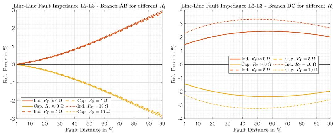
Figure 75: Relative measurement error in branch CD1 or CD2 and AB1 and AB2 for L-L fault, for inductive and capacitive operation of the SSSC and different  $R_f$
