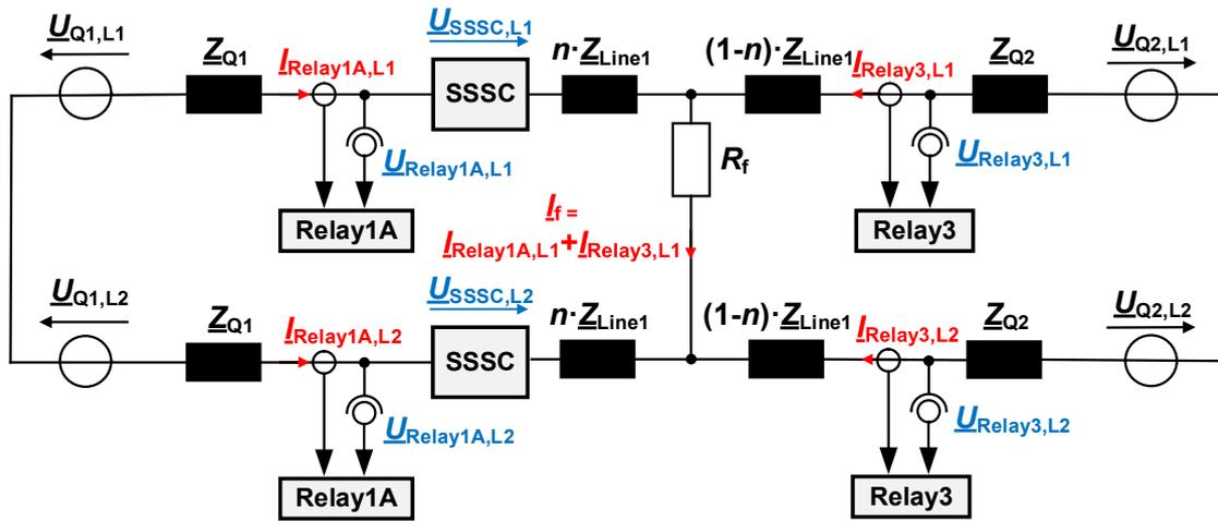
Figure 40: Equivalent circuit L1-L2 of a two-phase fault (L-L), based on Figure 37 while considering the fault resistance  $R_f$  and double infeed
