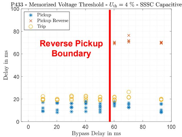
Figure 90: Pickup, pickup reverse and trip signals for P433 for memorised voltage threshold  $U_{th} = 4\%$  in dependency of the bypass delay
