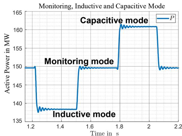
Figure 33: Load flow control by SSSC
