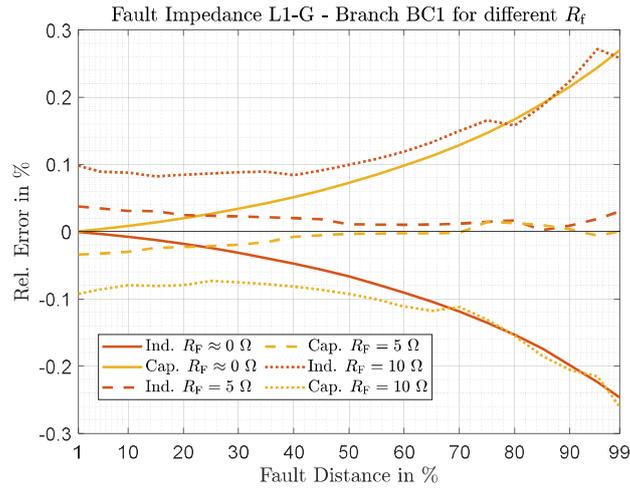
Figure 72: Relative measurement error in branch BC1 for L-G fault, for inductive and capacitive operation of the SSSC and different  $R_f$
