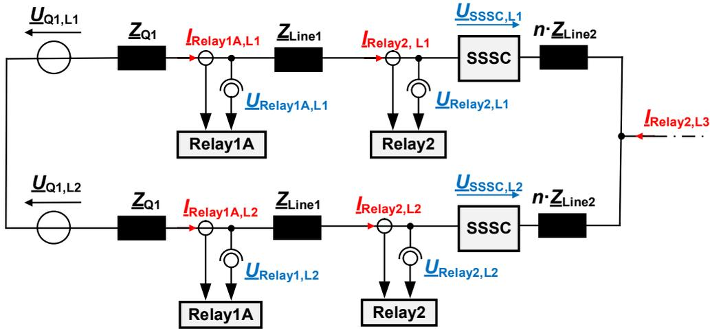
Figure 46: Equivalent circuit L1-L2 of a three-phase fault (L1-L2-L3), based on Figure 45 while neglecting the fault resistance  $R_f$
