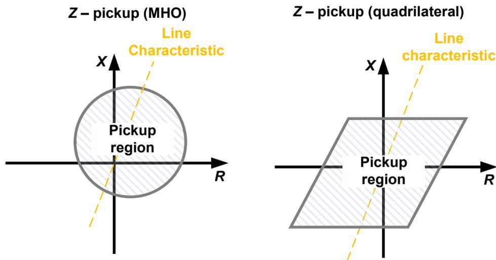
Figure 6: Z – Pickup with MHO- (left) and quadrilateral characteristics (right) based on [4]
