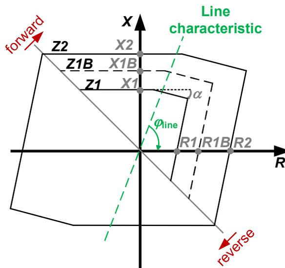
Figure 7: Example structure of a quadrilateral tripping characteristic based on [3,5]
