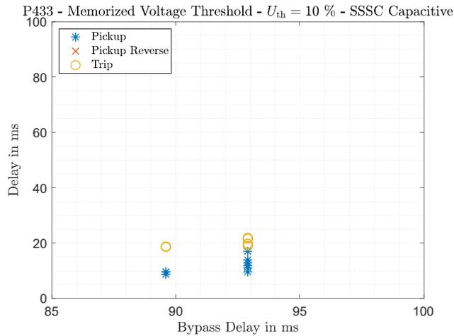
Figure 88: Pickup and trip signals for P433 for memorised voltage threshold  $U_{th} = 10\%$
