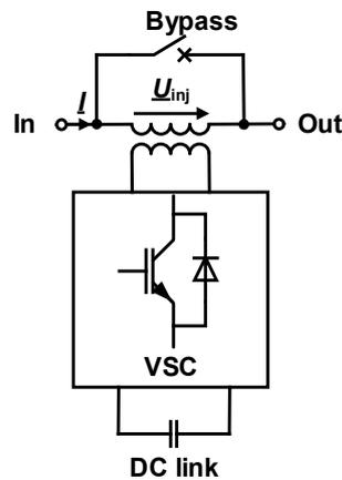
Figure 17: Static Synchronous Series Compensator (SSSC) based on [10]
