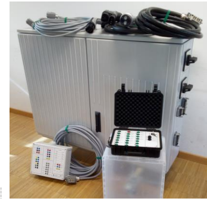
Fig.1: measurement distribution board
