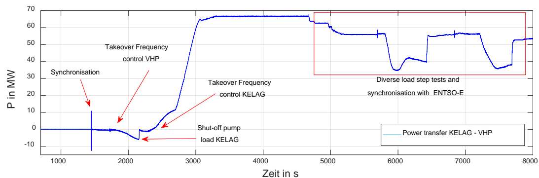
Figure 2: Measured active power transfer between two island after synchronization from 2017 grid restoration test Kärnten
