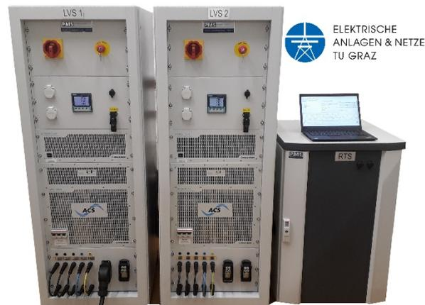
Abbildung 1: Power Hardware-in-the-Loop System
