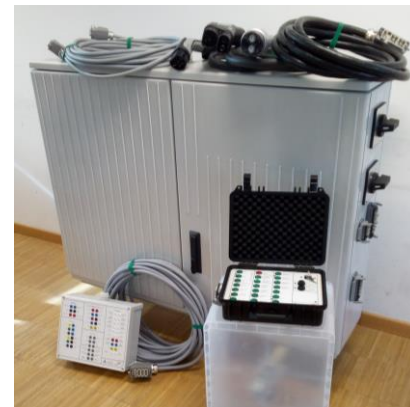
Fig. 3: Measurement distribution box
