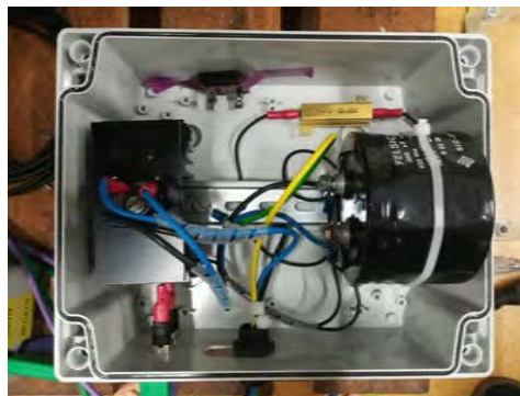
Figure F.2: Figure of the full-wave rectifier and the smoothing capacitor with parallel resistor R 1 .
