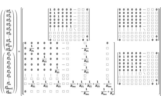
$$\begin{pmatrix} \underline{U}_{L,S}^{A} \\ \underline{I}_{L,S}^{A} \end{pmatrix} = \begin{bmatrix} E_{n} & N_{n} \\ A_{n} & E_{n} \end{bmatrix} \begin{pmatrix} \underline{U}_{L,S}^{E} \\ -\underline{I}_{L,S}^{E} \end{pmatrix}$$
