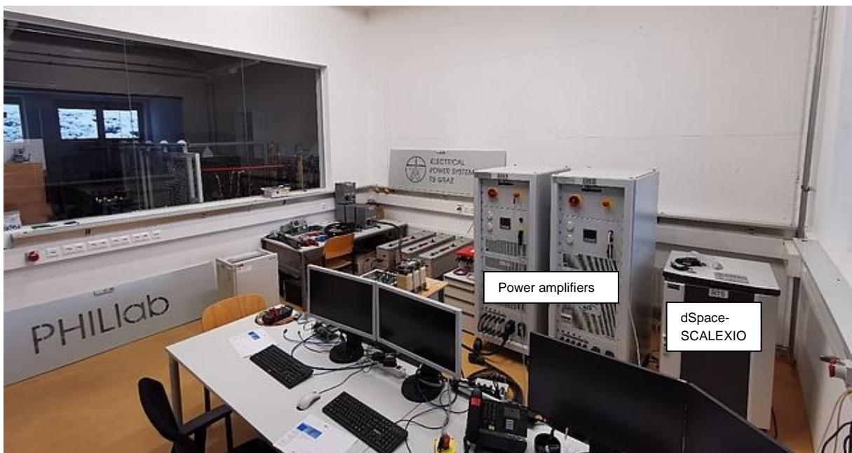
Figure 8: PHIL lab equipment at the institute of electrical power systems, TU Graz [7].
