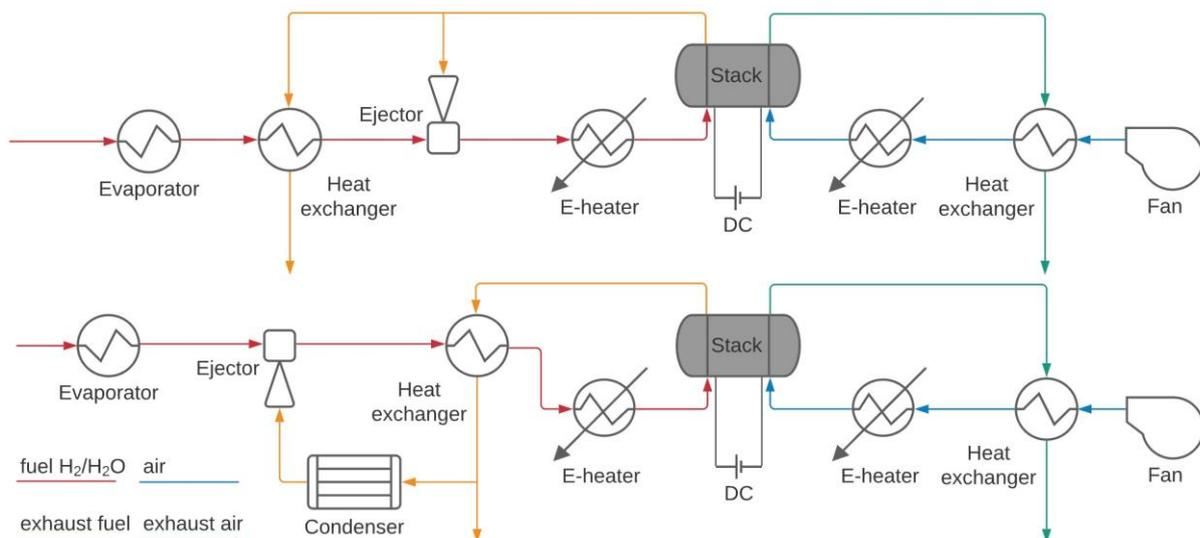
Figure 1 Basic system layouts, upper illustration with hot- and lower with cold-gas-recirculation
