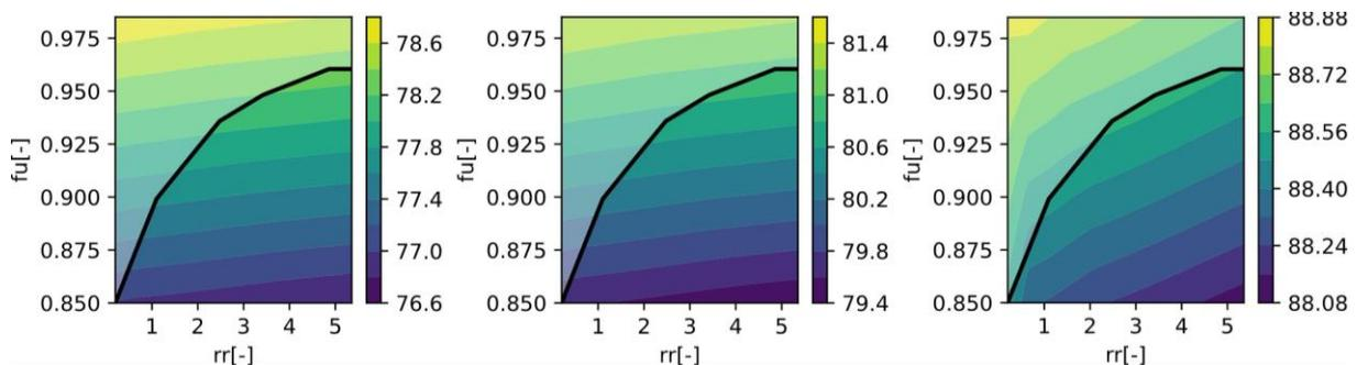
Figure 2 Dependency of system efficiency on the parameters volumetric recirculation rate ( $rr$ ) and fuel utilization ( $fu$ ) for (left) the case of providing high temperature and evaporation heat electrically, (middle) with recovery of waste heat from the air stream, (right) with recovery of waste heat and external heat source providing exergy for evaporation, greyed above black line: non-allowed stack operation
