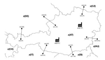
Figure 1:Concept of zones where each country is its own zone z. The dynamic set gz(g,z) represents the generators within a zone and the dynamic set lbz(i, j, c) contains all lines between different zones.
