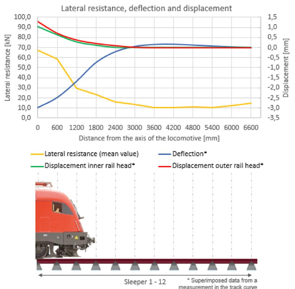
Fig. 2: Superimposition of data from track curve and transverse displacement resistance measurement
