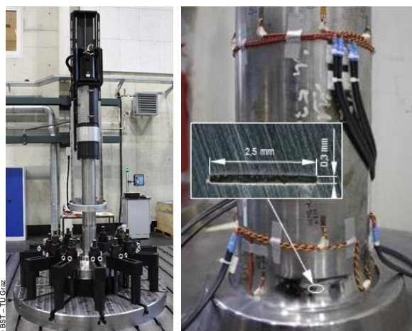
Crack propagation test at a railway axle
