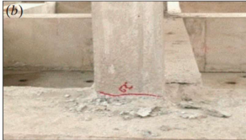
Typical crack modes of the CIS RAC frame
