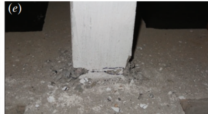
Typical crack modes of the precast RAC frame
