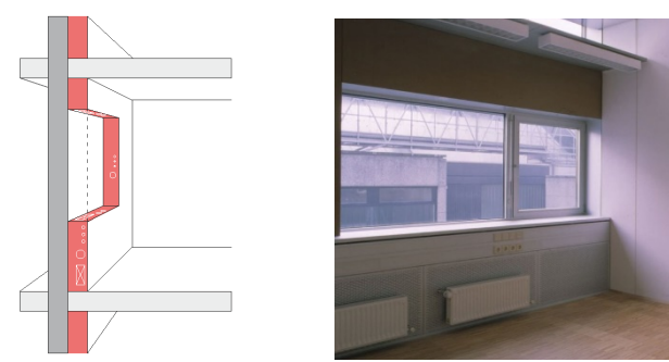
Cable arrangement in front of vertical building components
