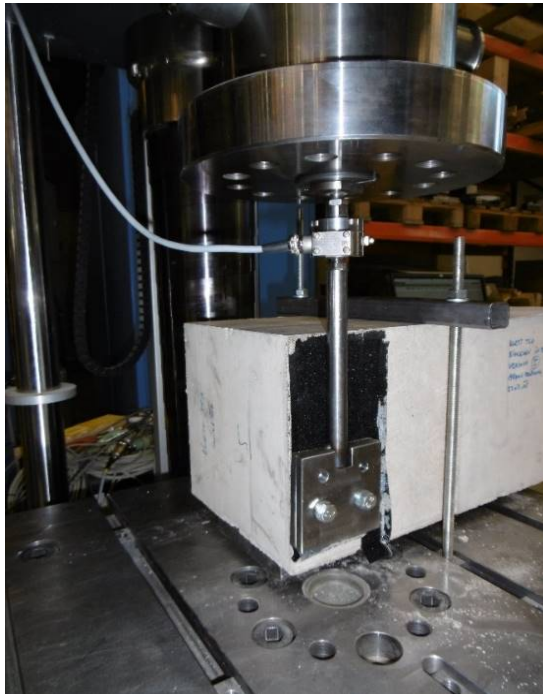
Experimental Setup of the peeling and pull-out tension test with Loop-Fastener. The width of the test strip is 5 cm.
