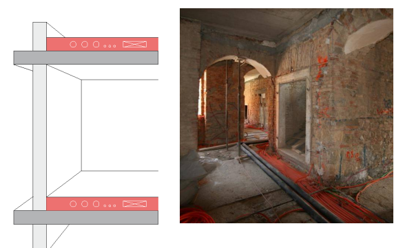
Cable arrangement above horizontal building components
