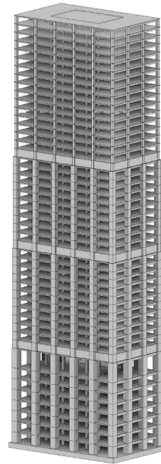
T2 Tubed mega frame + outriggers
