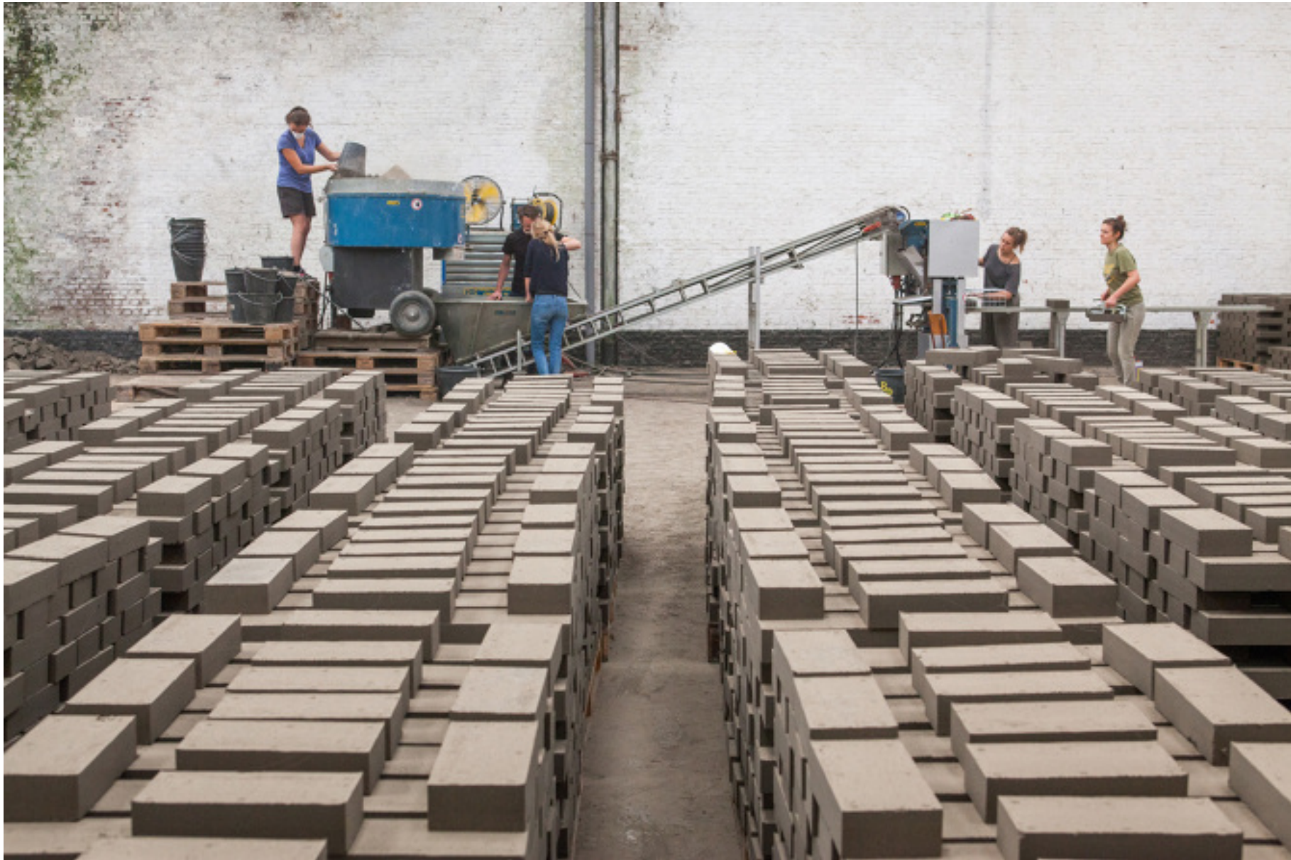
Bioclass, Edegem, 2018 Load-bearing compressed earth bricks ( BC architects & studies )
