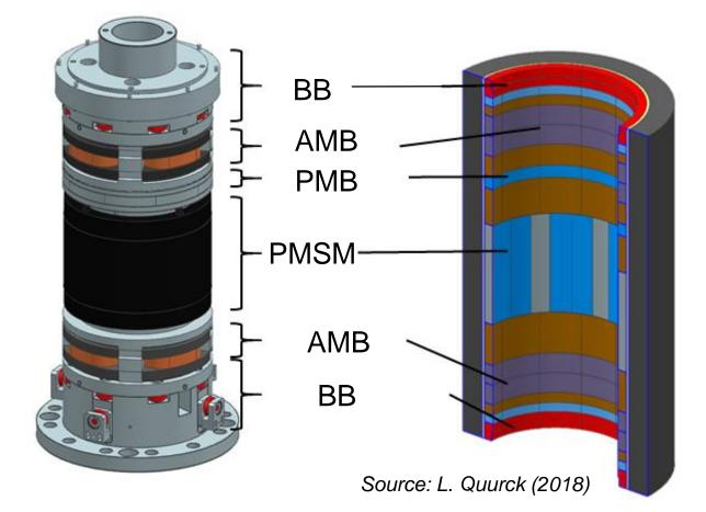
Innovation through highly integrated outer rotor
