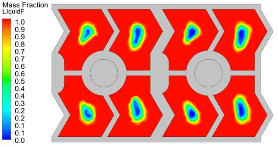
T<sub>fusion</sub> = 23°C Heating flow at 35°C
