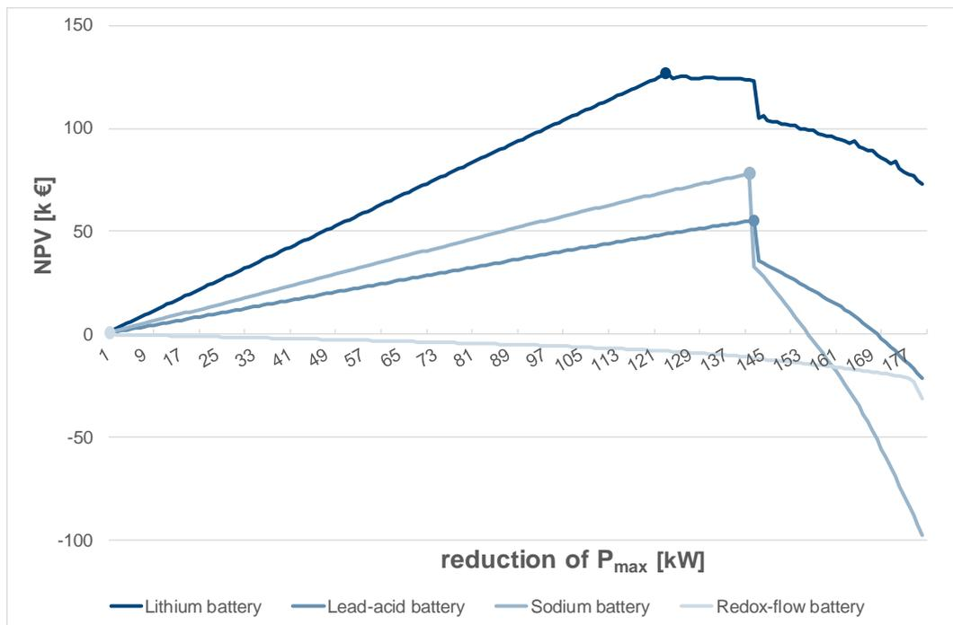
Figure 2 NPV of the energy storage technologies for the reduction of  $P_{max}$  for peak shaving
