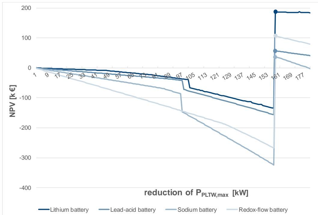
Figure 3 NPV of the energy storage technologies for the reduction of  $P_{PLTW,max}$  for atypical grid usage
