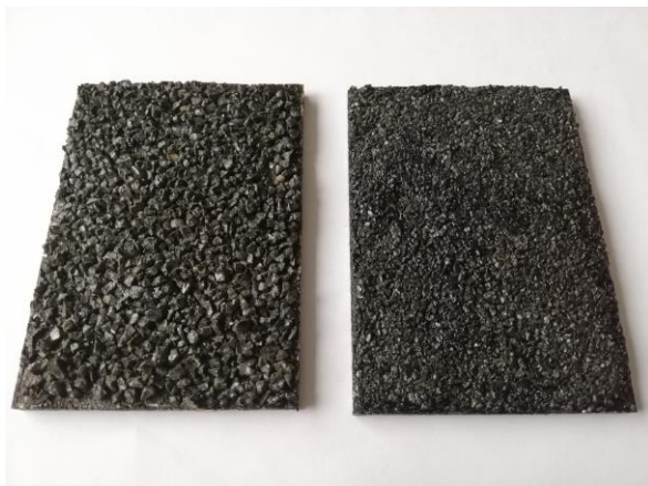
Figure 5. Aluminium foam samples (dimensions 105 x 75 x 6 mm) coated by bitumen-based matrix composite reinforced by fine-grained basalt granules (size of basalt granules: 2 – 4 mm – left, 1 – 2 mm – right).
