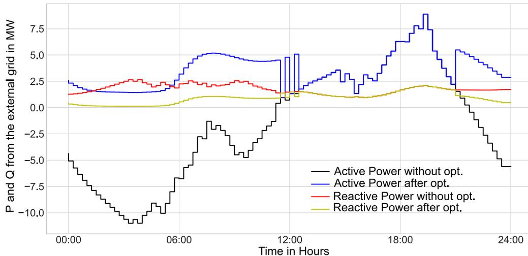
Figure 7: Active and reactive power from the external grid
