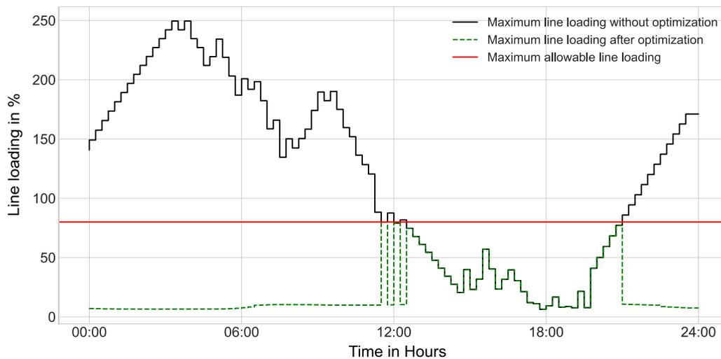
Figure 3: Line loading before and after optimization
