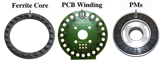
Fig. 2. Prototyped PCB winding motor components.
