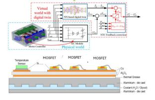
The power switch of a phase-leg is not integrated in a power module but rather consists of 4 discrete switching elements whereas every switching element is built by 3 power switches in parallel. Thus, the system consists in total of 36 power switches for the three phases, which are distributed on a single heat sink and the individual junction temperatures are challenging to predict.
