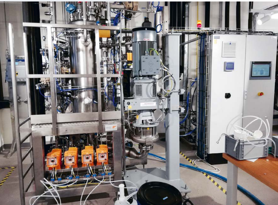
Figure 3: Pilot gas bioreactor at 300 L volume capacity.
