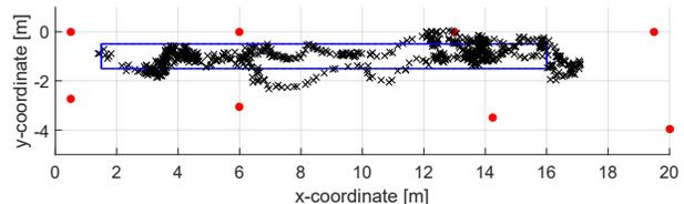
Fig. 6: Exemplary result. The red circles are the sensor positions. The blue line indicates the ground truth (walking with 0.5 m/s, starting point is top right in clockwise direction). The black crosses are the position estimations.
