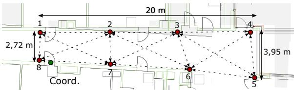
Fig. 4: Measurements of the testbed. The red circles are the sensor nodes, the dashed line the streams.
