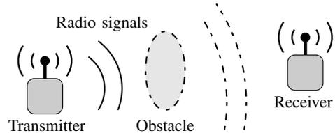
Fig. 1: Radio propagation obstructed by an obstacle.
