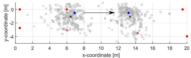
Fig. 5: The blue circle is the ground truth, the black cross the position estimation. The gray circles are the particles.
