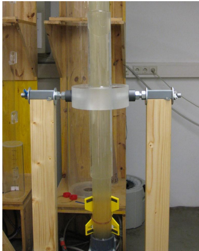
Figure 4.17: Assembly for holding the settling column
