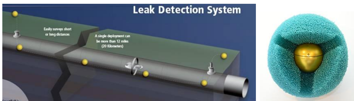
Figure 1.10: Smart Ball® Injection Process (Pure Technologies)
