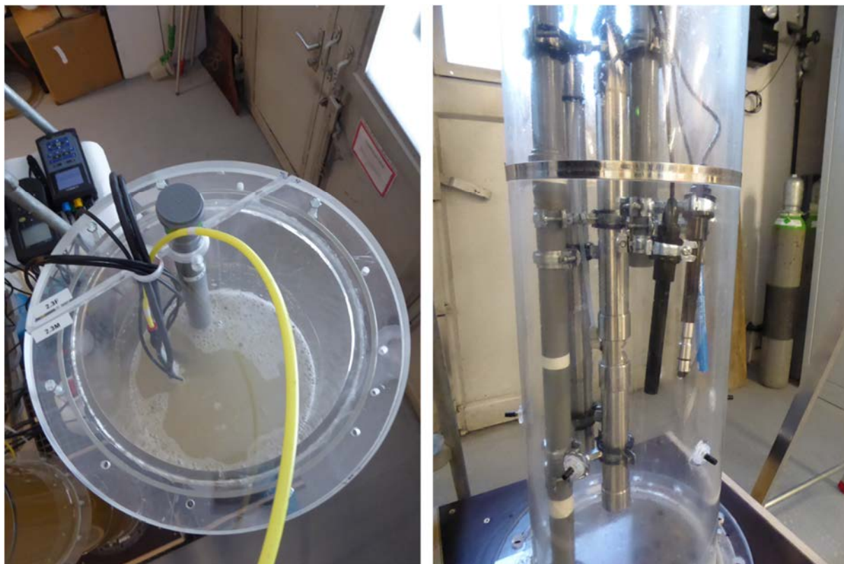
Figure 2-17: Split top lid (left) and mounting system after reactor discharge (right)
