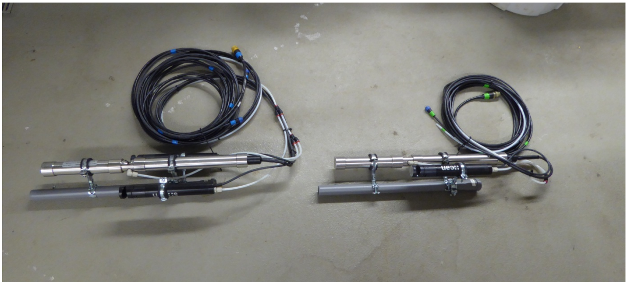
Figure 2-16: Outer cladding tube elements, probes mounted with pipe clamp systems
