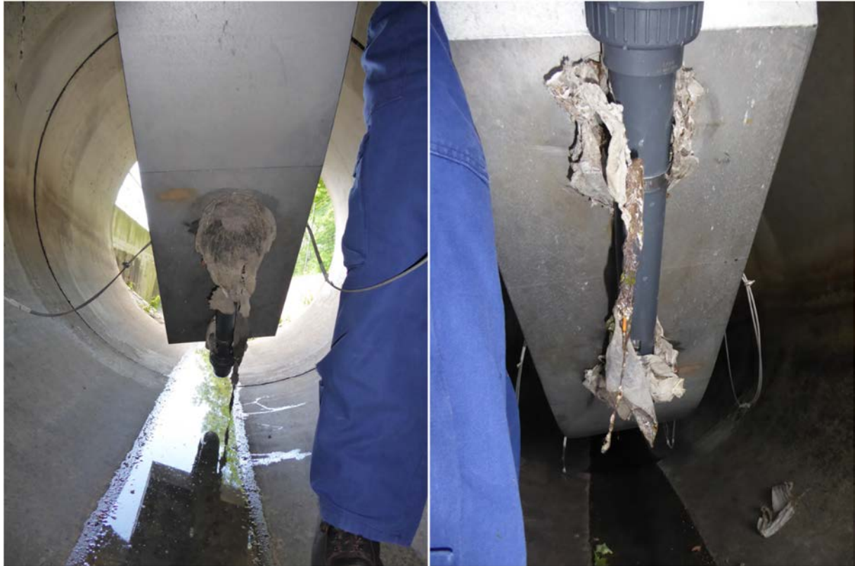
Figure 2-25: Clogging of the cladding tube in which the spectrometer probe is installed after an overflow event (Images: Hofer, 2016)
