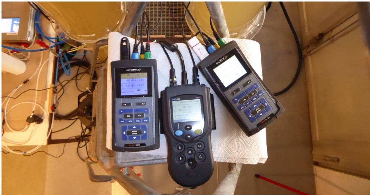
Figure 2-4: Applied control units for secondary probes designed for laboratory use
