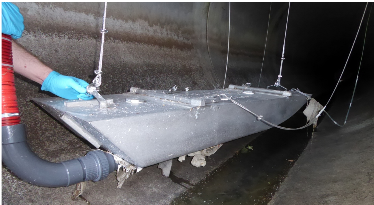
Figure 2-24: Side view of the floating pontoon in Graz-WWTP-CSO where the spectrometer was installed after an overflow event (Image: Hofer, 2016)
