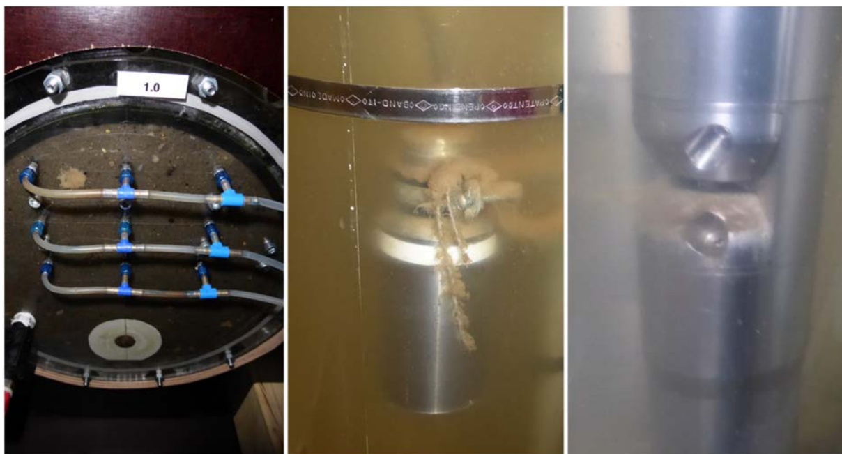
Figure 3-1: Sediment at the bottom of a GEN 2-reactor (left), on the equipment (middle) and around the measurement window of a spectrometer probe (right)
