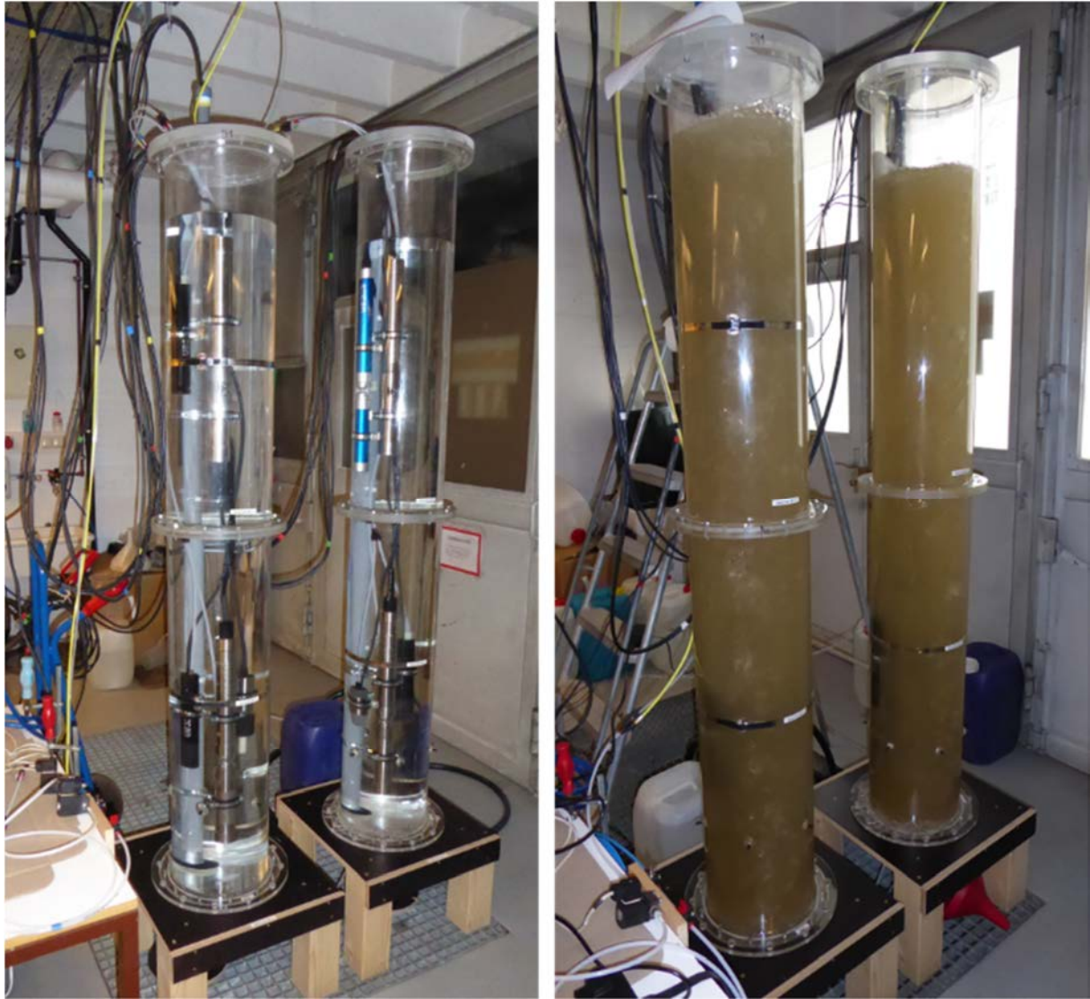
Figure 2-13: Reactors of GEN 2 with test configuration during the final stress test (left) and during an agitation period (right)
