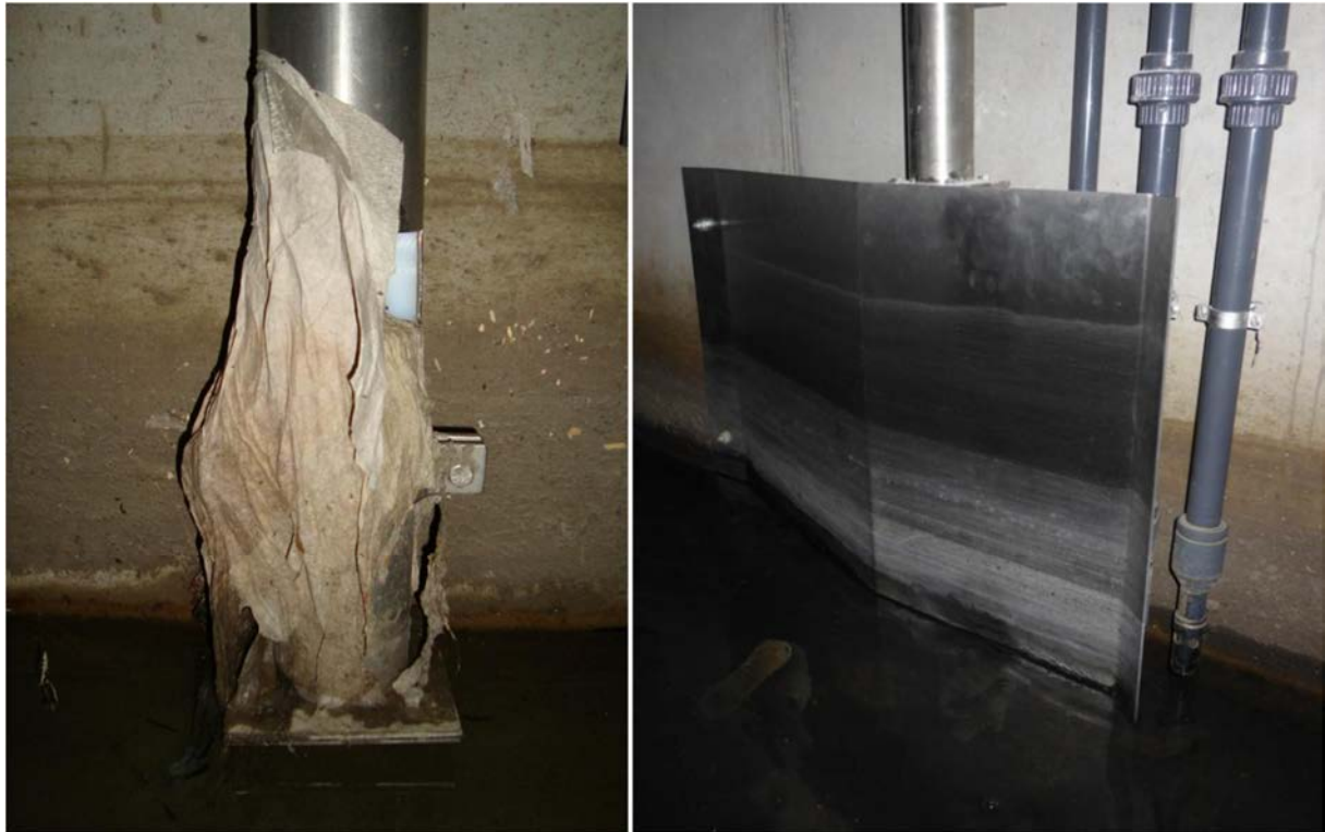
Figure 2-6: Clogged spectrometer probe (left) before the installation of a sheet metal cover (right) (Images: Graz University of Technology, 2014)
