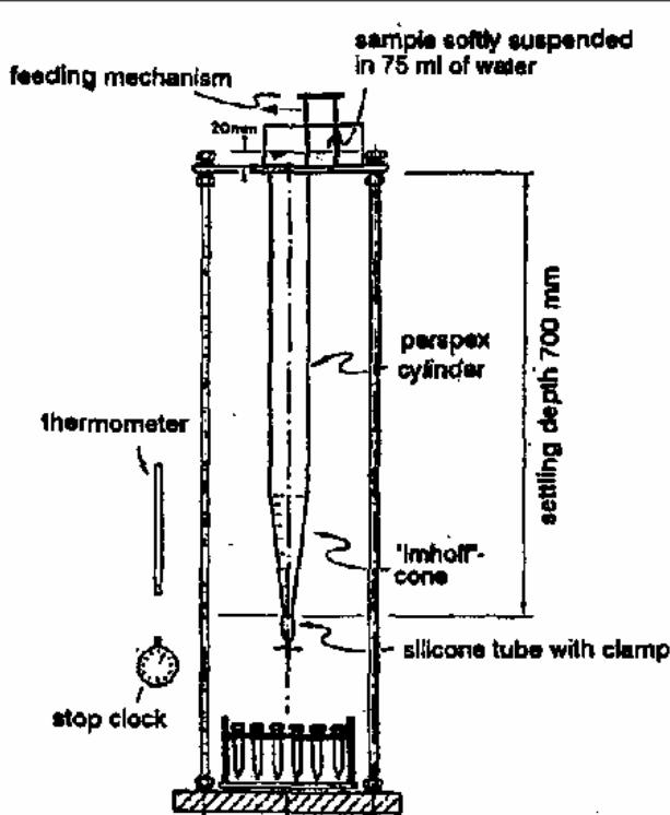
**Figure 10 Settling apparatus german protocol (Brombach, 1990)**
