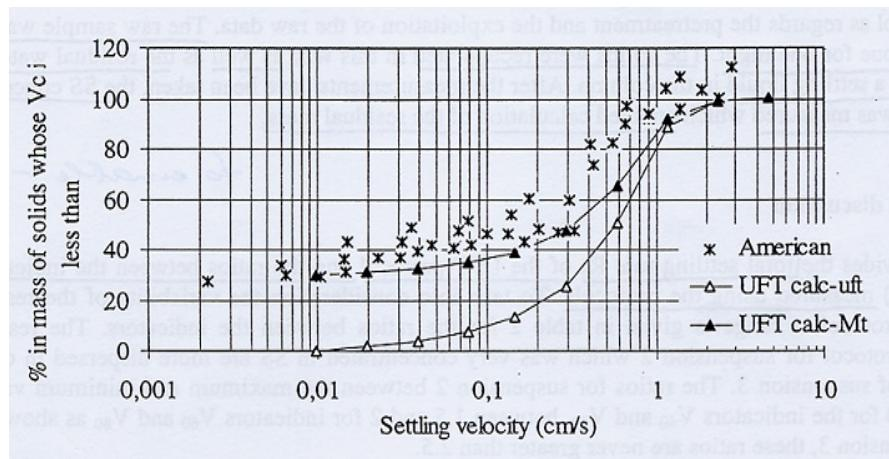
**Figure 14 Settling velocity curves measured with UFT protocol and the American method (Chebbo, 1992)**
