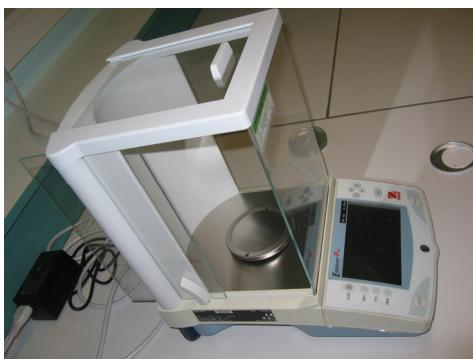
**Figure 46 Weighting of the filters**
