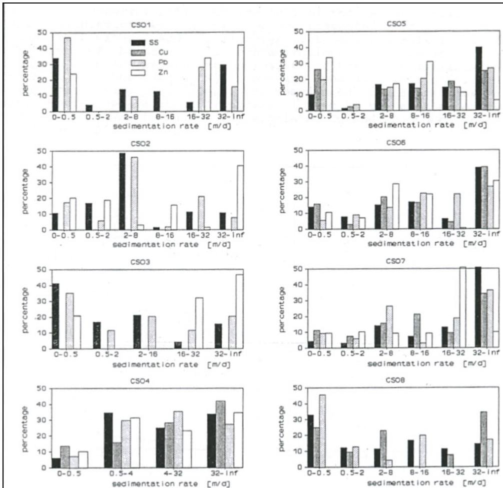
**Figure 7 Normalized distributions of sedimentation rates of SS and associated heavy metals Cu, Pb and Zn (Benoist and Lijklema, 1990)**
