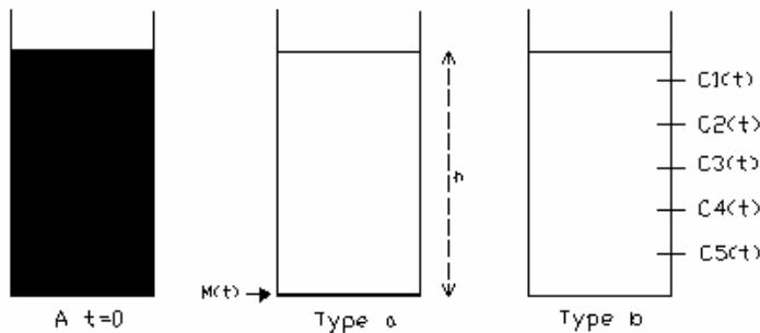
**Figure 3 Principle of the homogeneous suspension**
