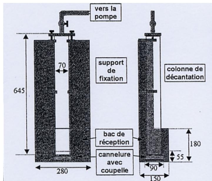
**Figure 12 Scheme of the breadboard construction, details of the column, details of the mixing vat, details of the groove:**
