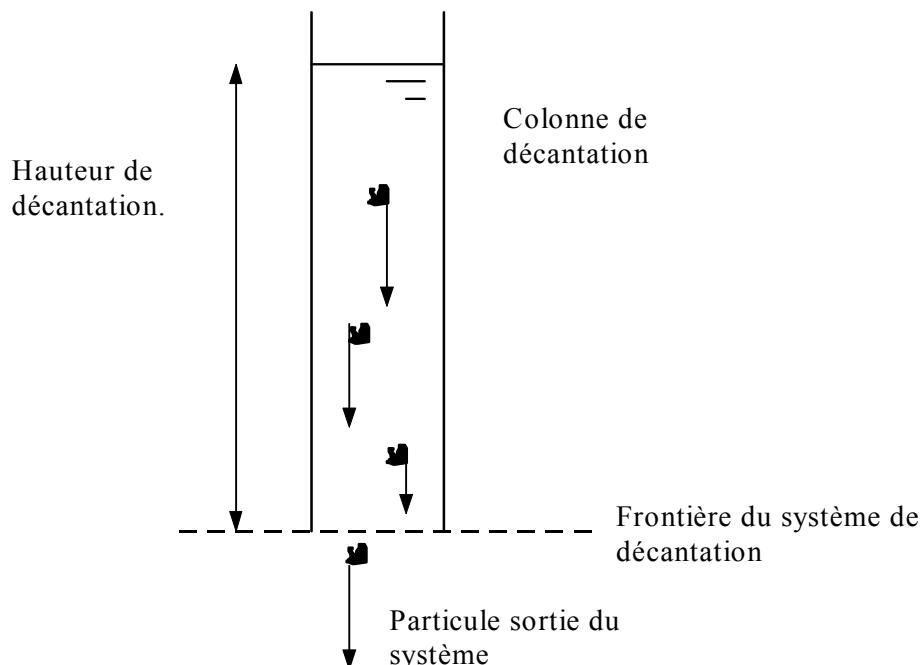
**Figure 4 Principle of the Cergrene settling column (in French)**
