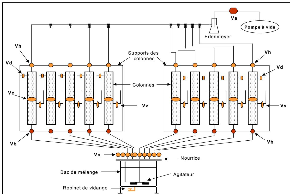
**Figure 5 Principle of the protocol Victor (Chebbo et al., 2003)**
