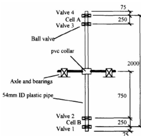
**Figure 8 Construction of the settlement velocity measurement column (Tyack, 1992), (values in mm)**
