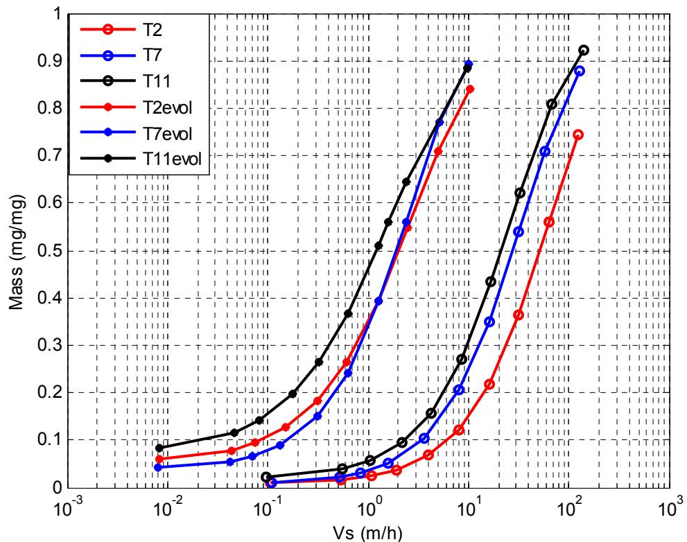
**Figure 85 Settling velocity curves at the time of the rain event and one month after**
