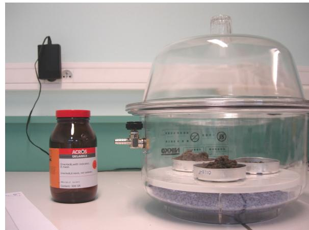
**Figure 49 Device of dessicant**
