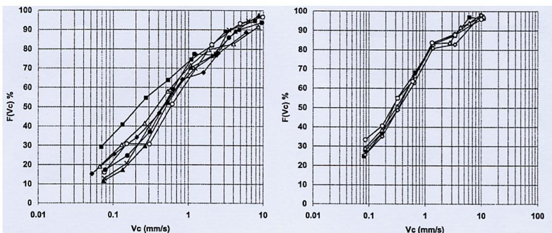
**Figure 21 Comparison of settling velocity grading curves measured with protocols Vicas and Vicpol**
