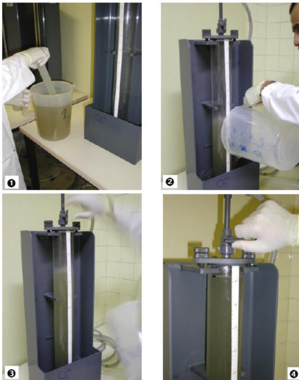
**Figure 43 Mixing of the sample and filling of the column**
