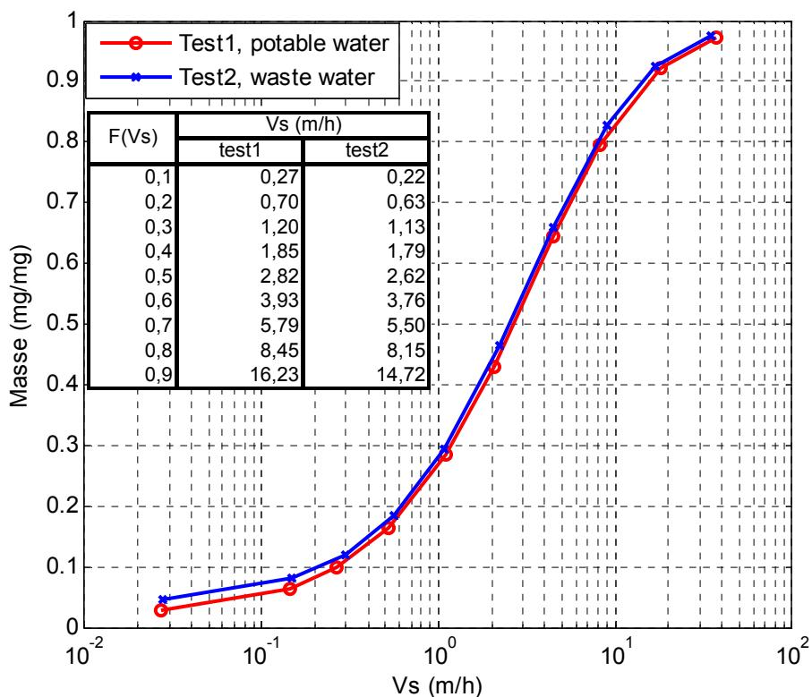
**Figure 60 Settling curves for Test1 and Test2**
