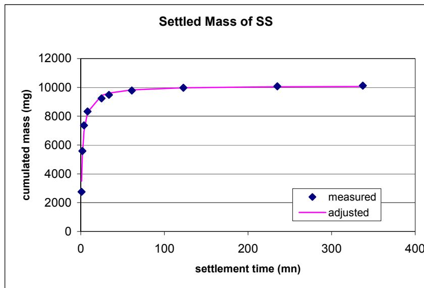
**Figure 32 Curve of the mass cumulated of solids elutriated according to time**
