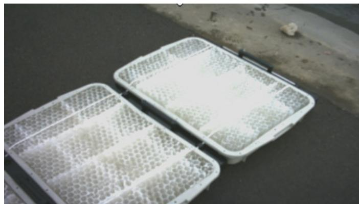
**Figure 28 Fixed settlement traps (plastic boxes and honeycomb structure)**
