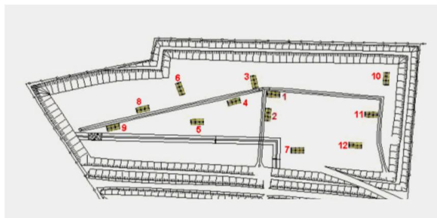
Figure 26 Plan with the 12 locations of settlement traps
