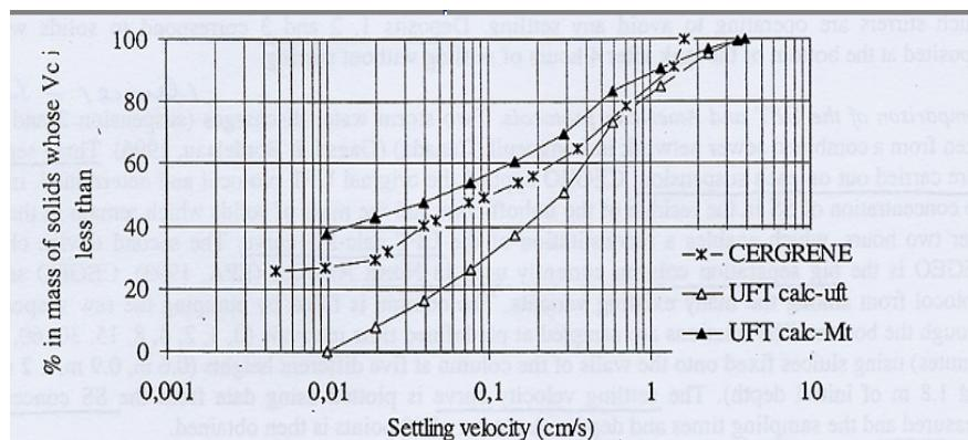
**Figure 13 Settling velocity curves measured with UFT protocol and the Cergrene method (Chebbo, 1992)**
