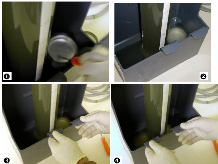
**Figure 44 Placing and changing of the cups**
