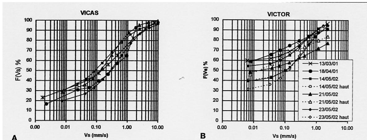
**Figure 18 Settling velocity distribution curves of the same sample measured with protocols Victor and Vicas (Chebbo, 1990)**
