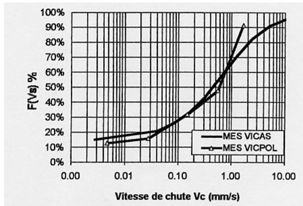
**Figure 20 Comparison of settling velocity grading curves measured with protocols Vicas and Vicpol**
