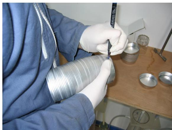
**Figure 40 Marking of the cups with the time steps of the settling intervals**
