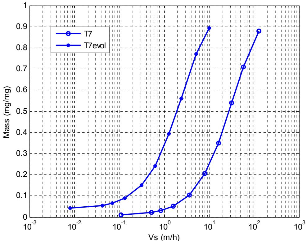
**Figure 87 Settling velocity curves of trap 7 at the time of the rain event and one month after**
