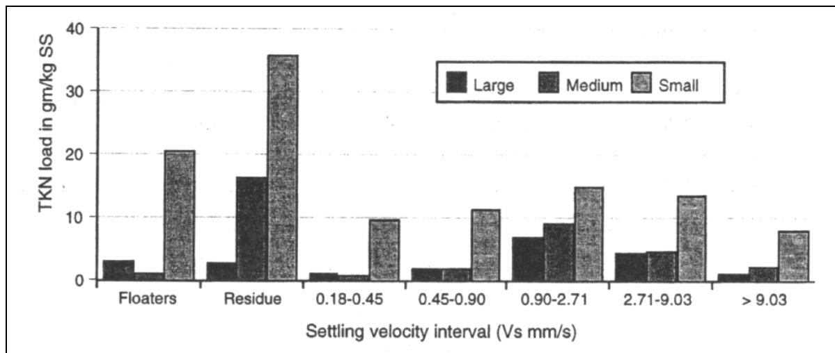
**Figure 17 Comparison of TKN distribution for different catchment area sizes**
