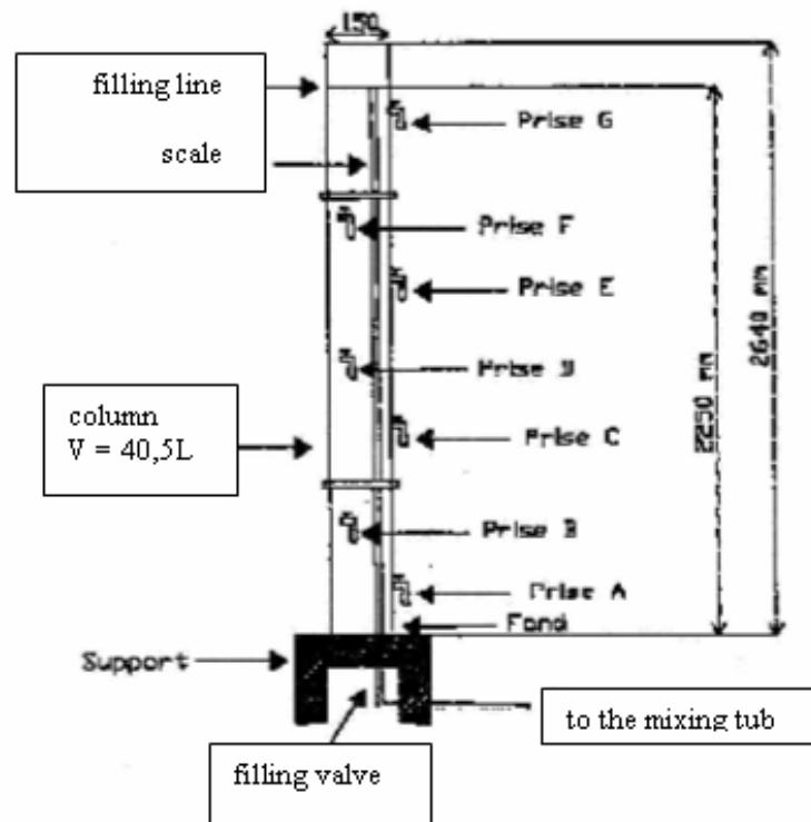
**Figure 11 Scheme of the American column applied by Gagné and Bordelau (1996)**
