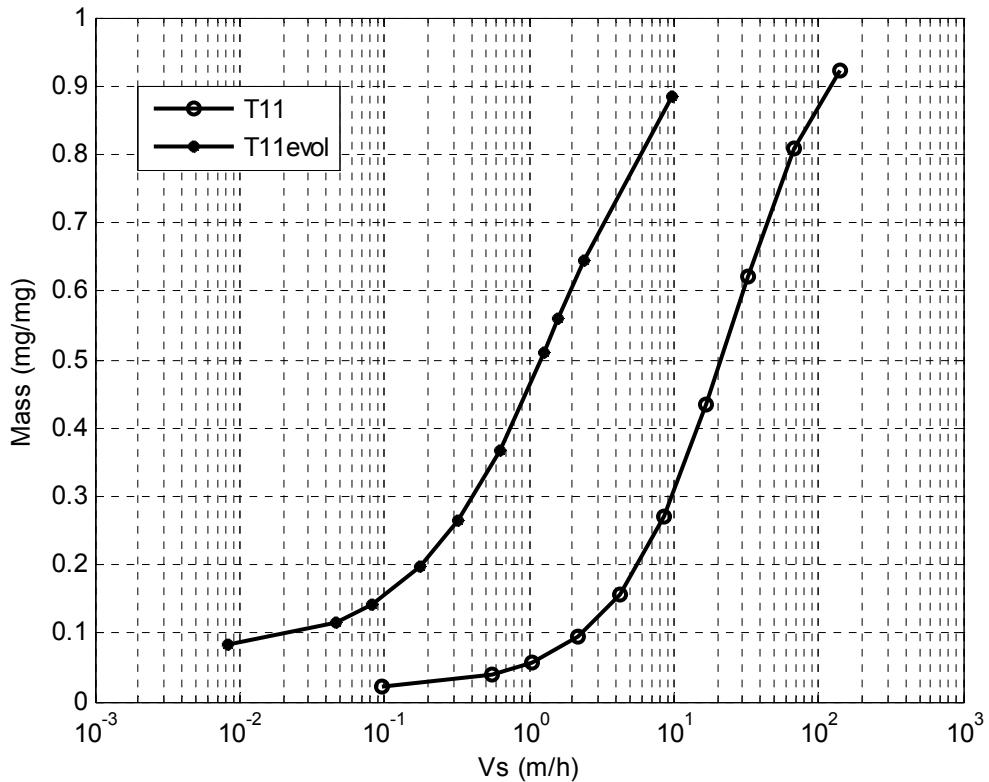
**Figure 88 Settling velocity curves of trap 11 at the time of the rain event and one month after**
