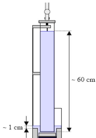
**Figure 42 Filling of the column**
