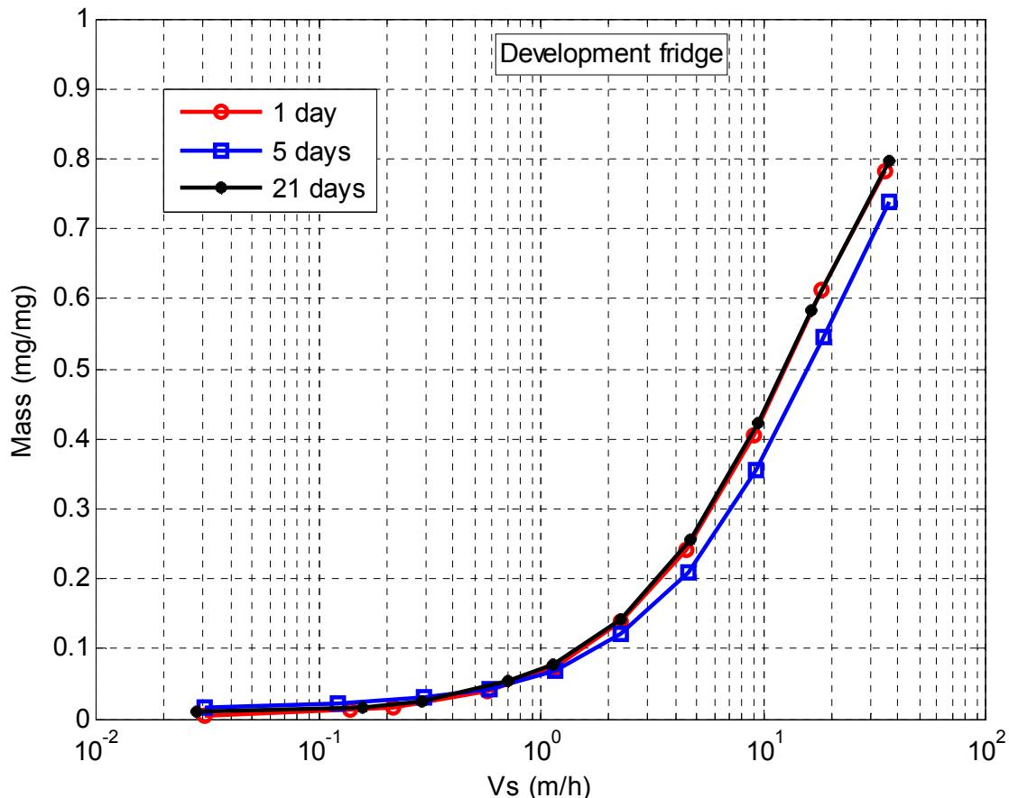
**Figure 61** Settling velocity curves from samples after different keeping time in fridge
