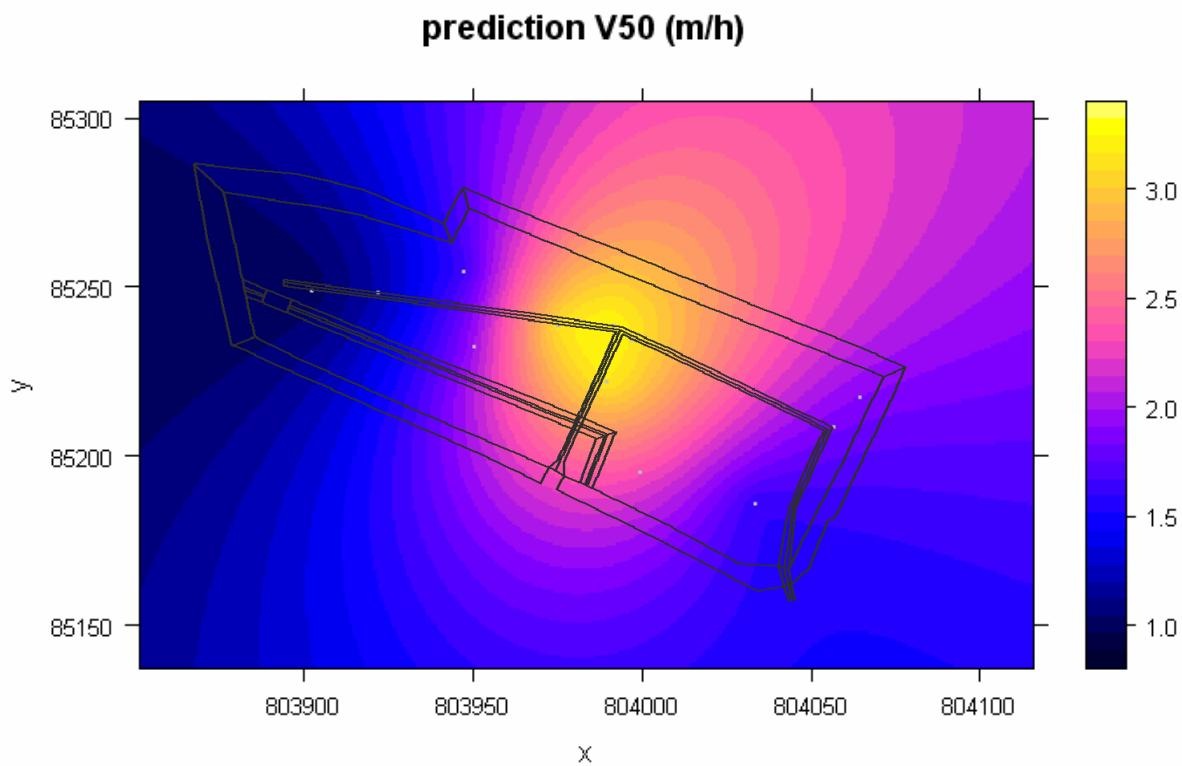
**Figure 57 Example of a result obtained by Kriging Interpolation**
