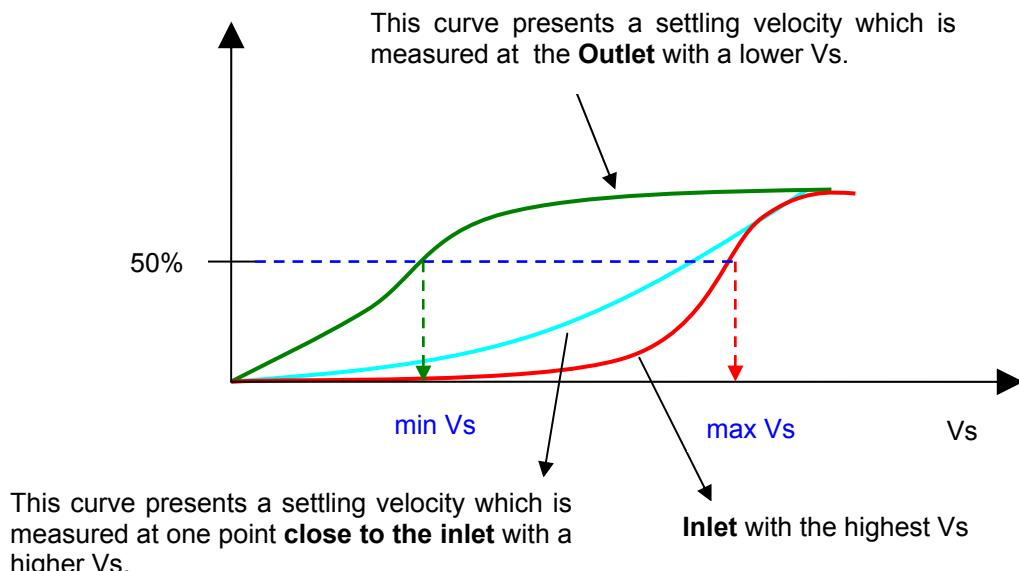
**Figure 83 Settling velocities according to different positions in the stormwater tank**
