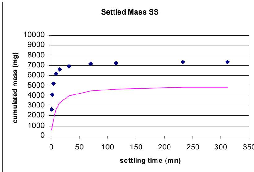
**Figure 52 Measured values by protocol Vicas with imprecise calibration of b, c and d**
