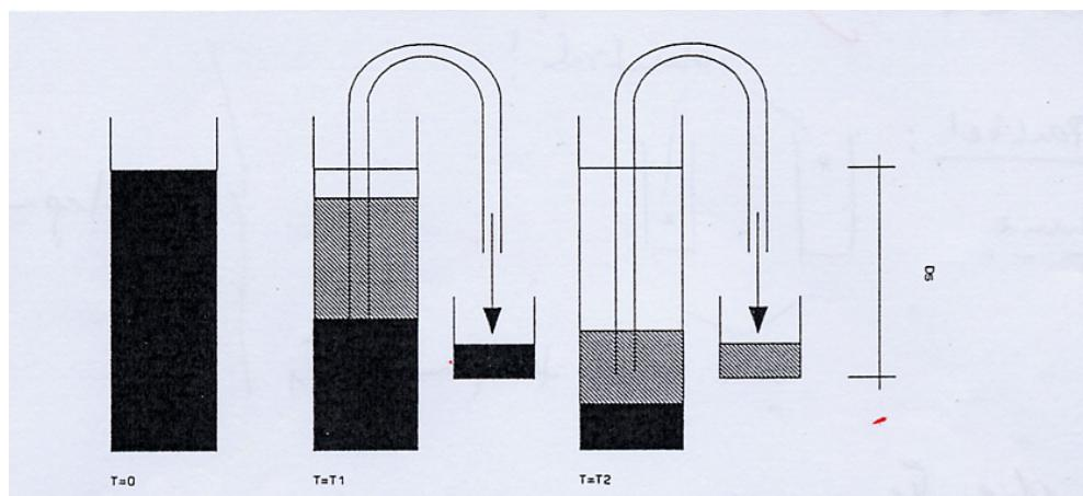
**Figure 6 Principle of measuring the distribution of sedimentation rates using settling tubes (Benoist and Lijklema, 1990)**
