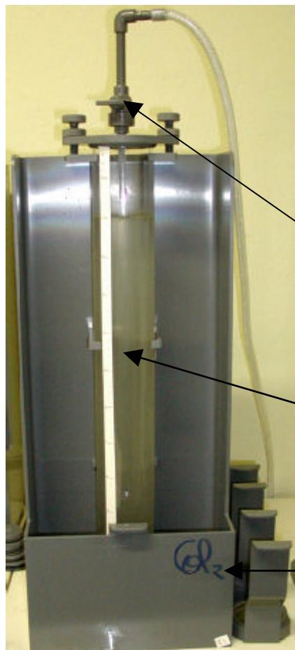
composed of a Plexiglass tube with an inner diameter of 70 mm and a height of 64 cm and provided with one scale graduated in cm indicating the distance from the bottom of the tube. The higher section of the column is connected to a rigid pipe provided with a valve allowing to seal the top of the column (Figure 35).
