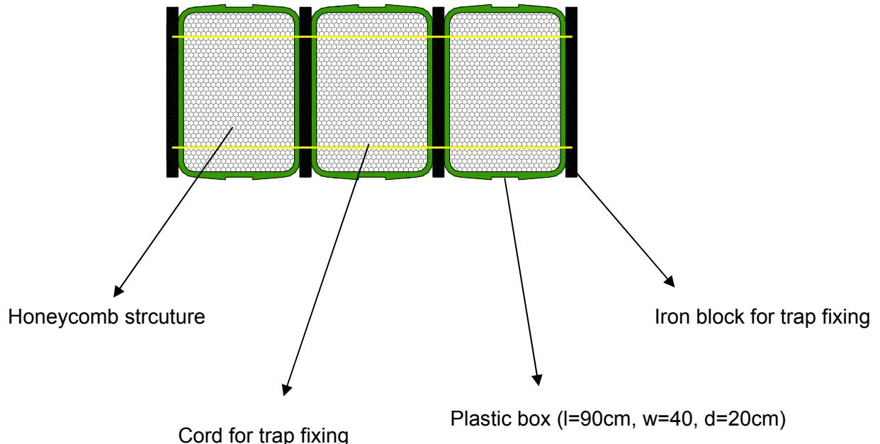
Figure 25 Plastic boxes with internal honeycomb structure
