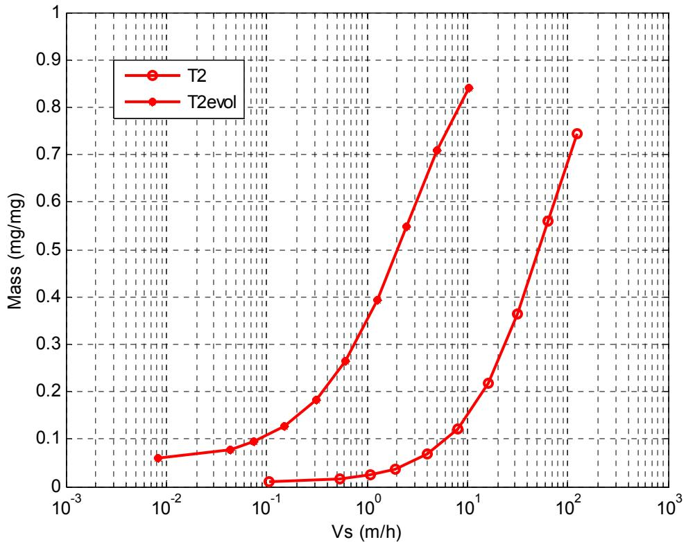
**Figure 86 Settling velocity curves of trap 2 at the time of the rain event and one month after**
