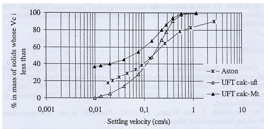
**Figure 15 Settling velocity curves measured with UFT protocol and Aston method (Chebbo, 1992)**
