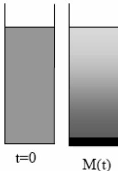
**Figure 31 Principle of the homogeneous suspension**
