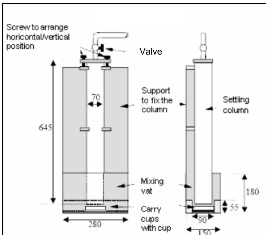
**Figure 38 Device for the settlement measurement for the protocol Vicas**
