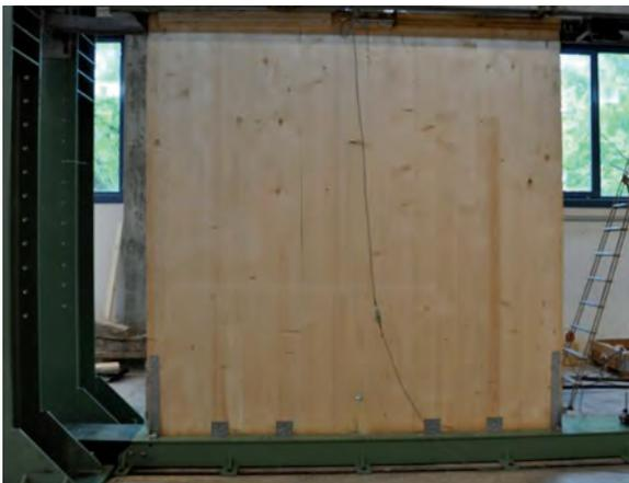
Fig. 3.3: *Cross-lam wall panels subjected to cyclic test (copyright IVALSA-CNR)*
