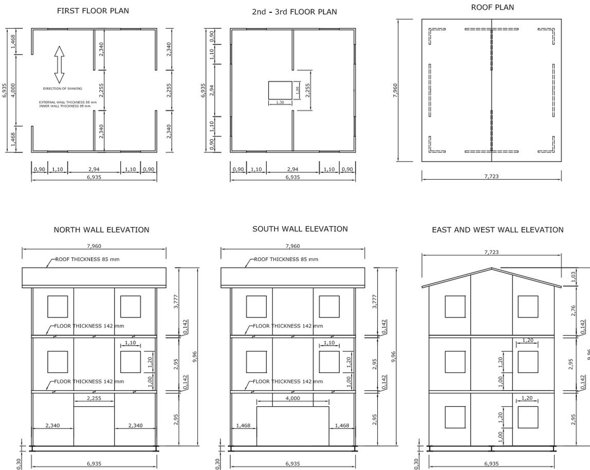
Fig. 3.3: Plan views and elevations of three-storey building in configuration C
