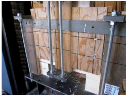
Fig. 5.14: Photo of experimental setup of a screwed joint with LVL strips between adjacent panels loaded under in-plane shear
