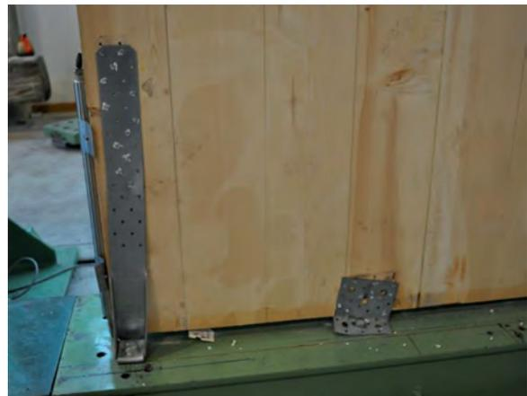
Fig. 3.4: *X-lam wall panel at the end of the cyclic tests, near to the failure condition (copyright IVALSA-CNR) - Note the hold-down and angle bracket on the left and right hand side, respectively.*
