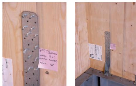
Fig. 4.1: Hold-down failure after Nocera Umbra 1.2g
