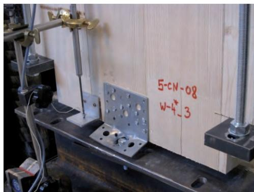
Fig. 5.7: Photo of experimental setup of an angle bracket loaded in tension
