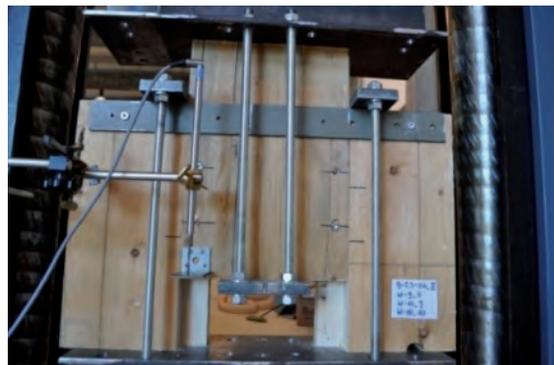
Fig. 5.12: Photo of experimental setup of an over-lapped screwed joint between adjacent panels loaded under in-plane shear
