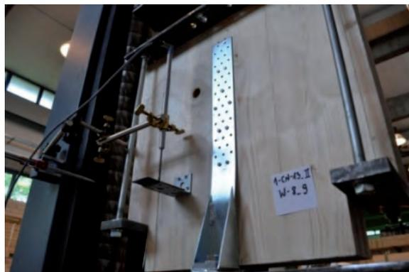
Fig. 5.2: Photo of experimental setup of a hold-down loaded in tension
