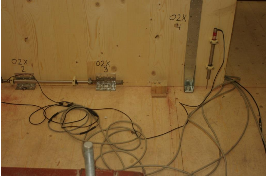
Figure 3.3: Wall uplift and sliding
