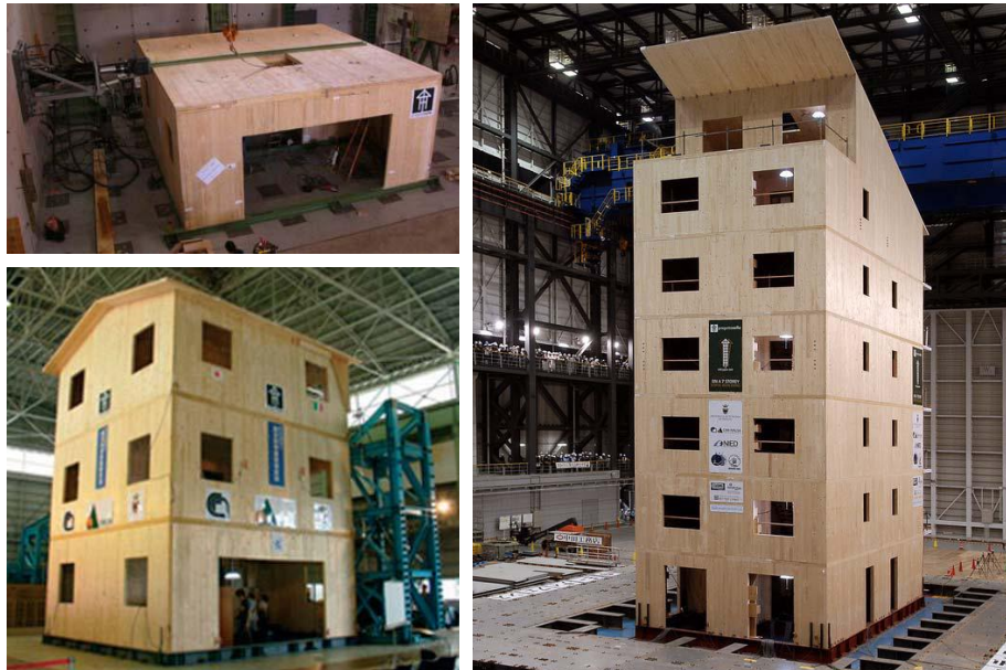
Figure 2.7: Tests in the context of the SOFIE project [8], [9], [10]
