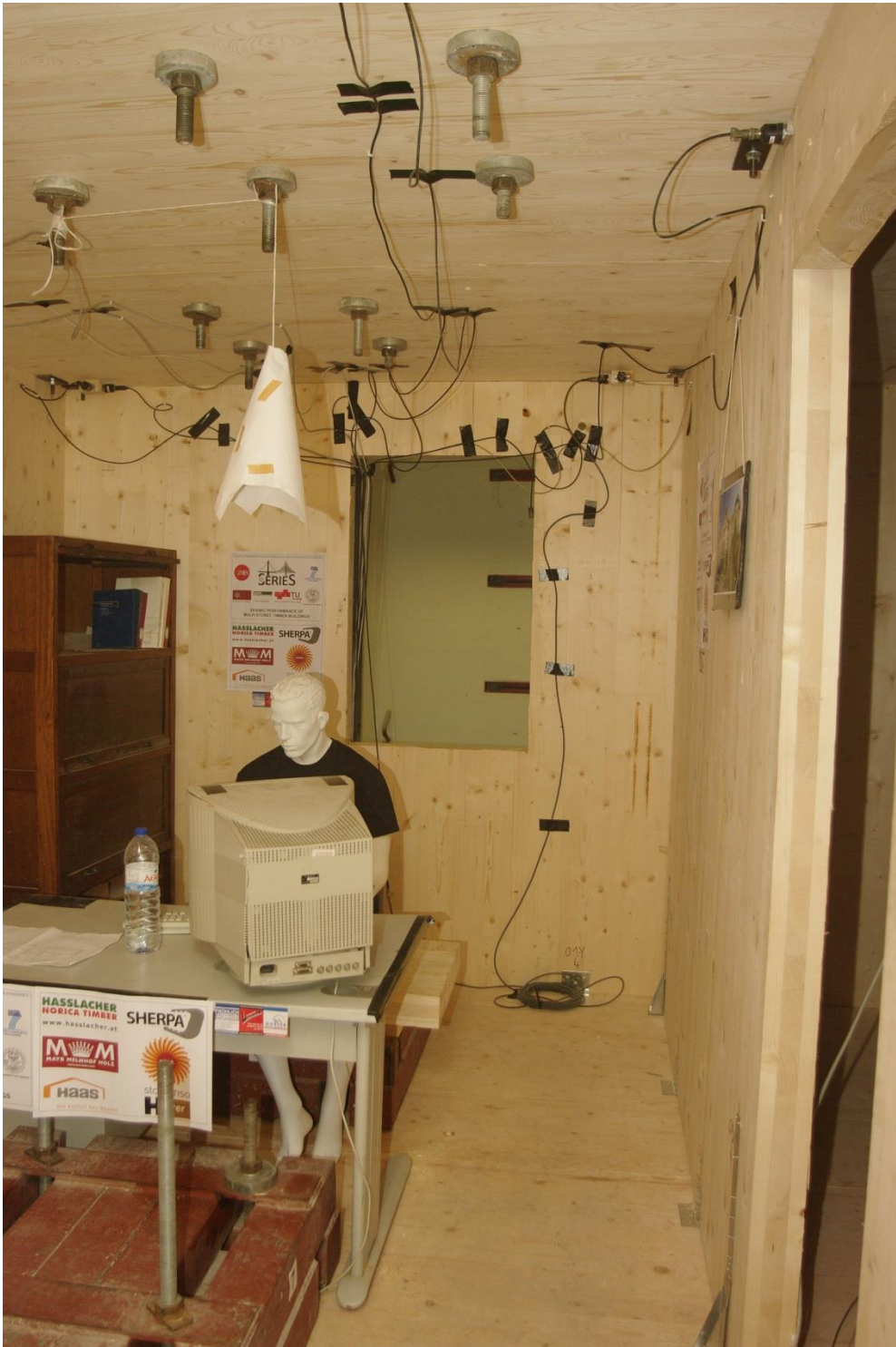
Figure 3.7: Several accelerometers placed on the monitored room
