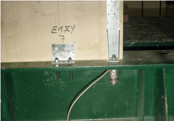
Figure 3.4: Details of annular load cells
