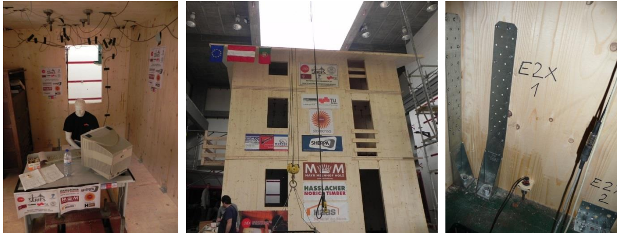
Figure 2.11: Full-scale shaking table test on a three storey CLT building
