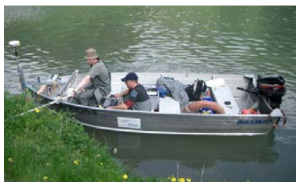
Stauraumvermessung mittels Echolot | Reservoir survey with Echolot
