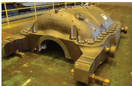
Figure 6: Outer Casing of Demonstration Turbine (Courtesy: Toshiba)
