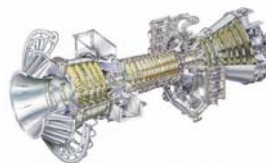
Fig. 13. The GE LM2500 (aeroderivative of the CF6-80C2). (Source: GE Power Systems)
