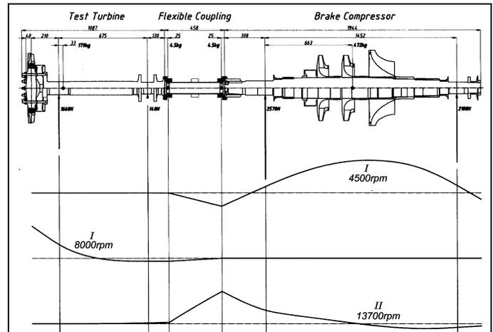
Figure 2: Test turbine and brake compressor bending modes
