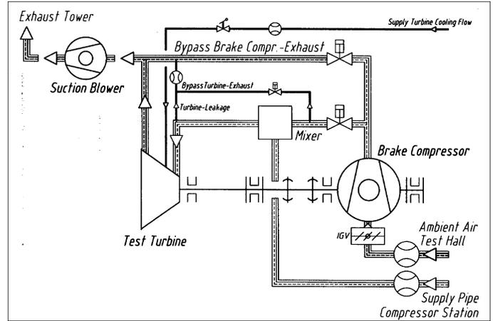
Figure 1: Schematic diagram of the turbine test rig
