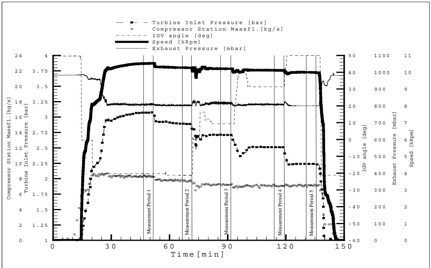
Figure 13: Time history of a typical test run
