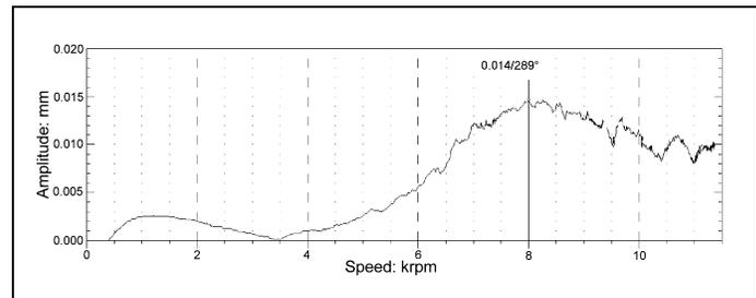
Figure 3: Movable bearing amplitude plot of a typical test run
