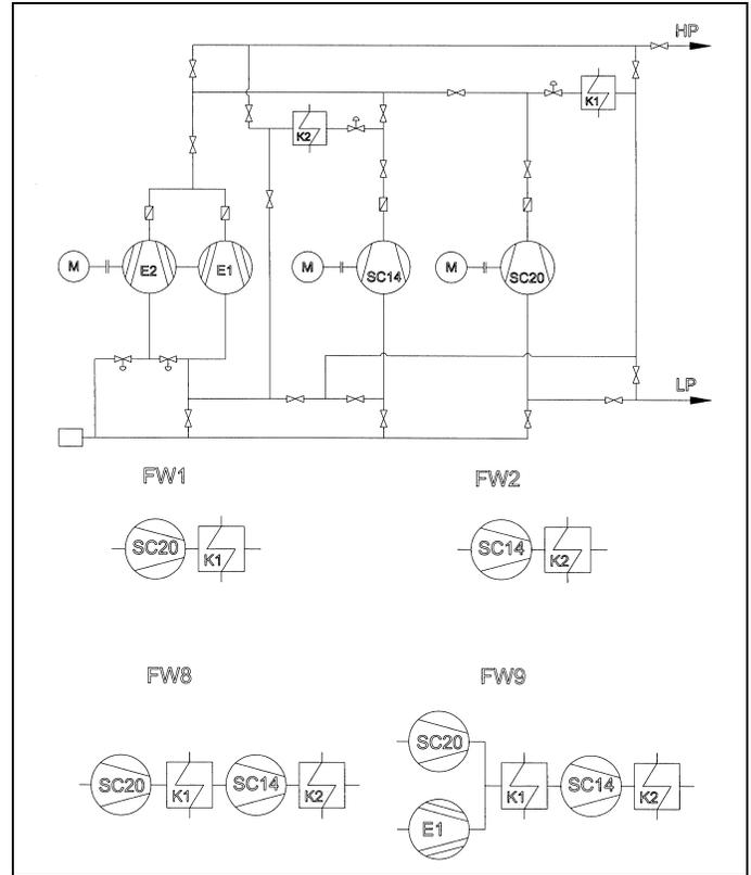
**Figure 4: Operational modes of the TTM compressor station**
