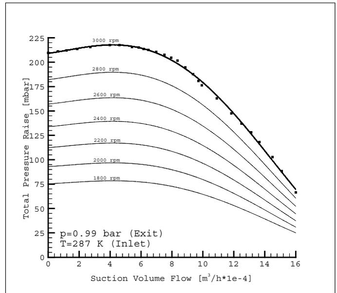
Figure 8: Suction blower characteristics
