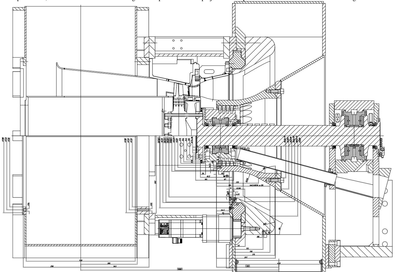
Fig.3 Transonic Test Turbine facility with TTM-Stage (upper half) and fitting dimensions for test stage inserts (bottom half)
