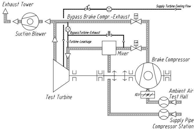
Fig. 1 Transonic Test-Turbine Facility flow scheme
