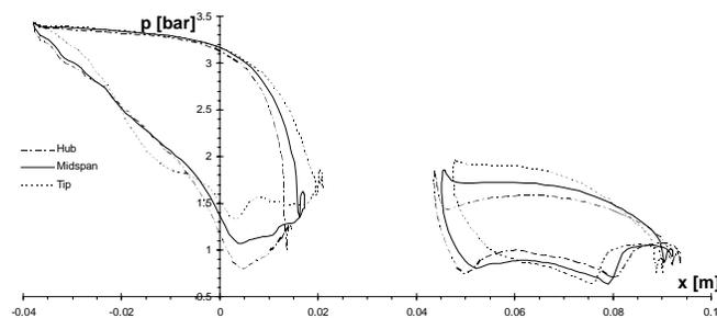
Fig. 11 Vane and blade surface Pressure distributions
