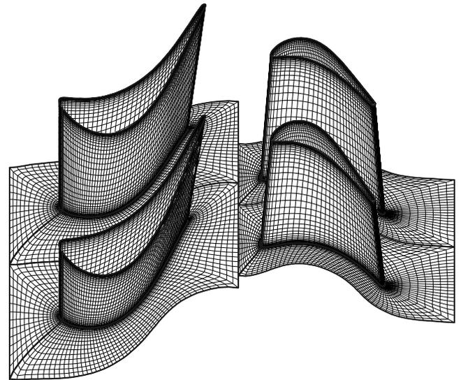
Fig. 5 Structured O-Type grid for 3D-viscous flow analysis (524288 cells in total)
