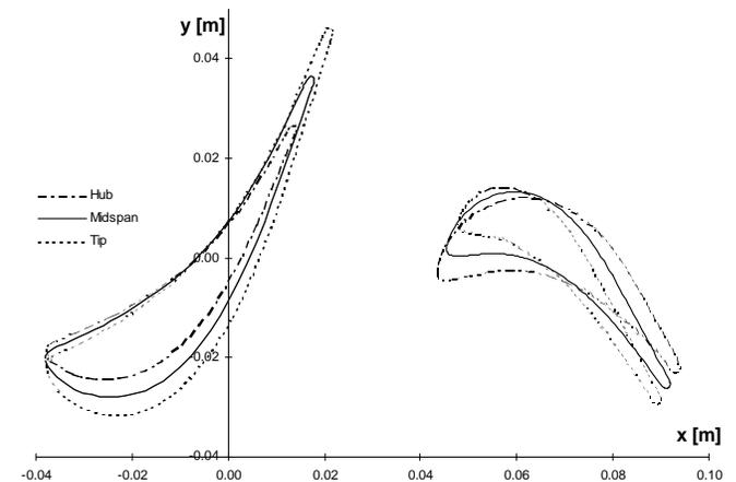
Fig. 9 Hub, Midspan and Tip sections of TTM-Stage
