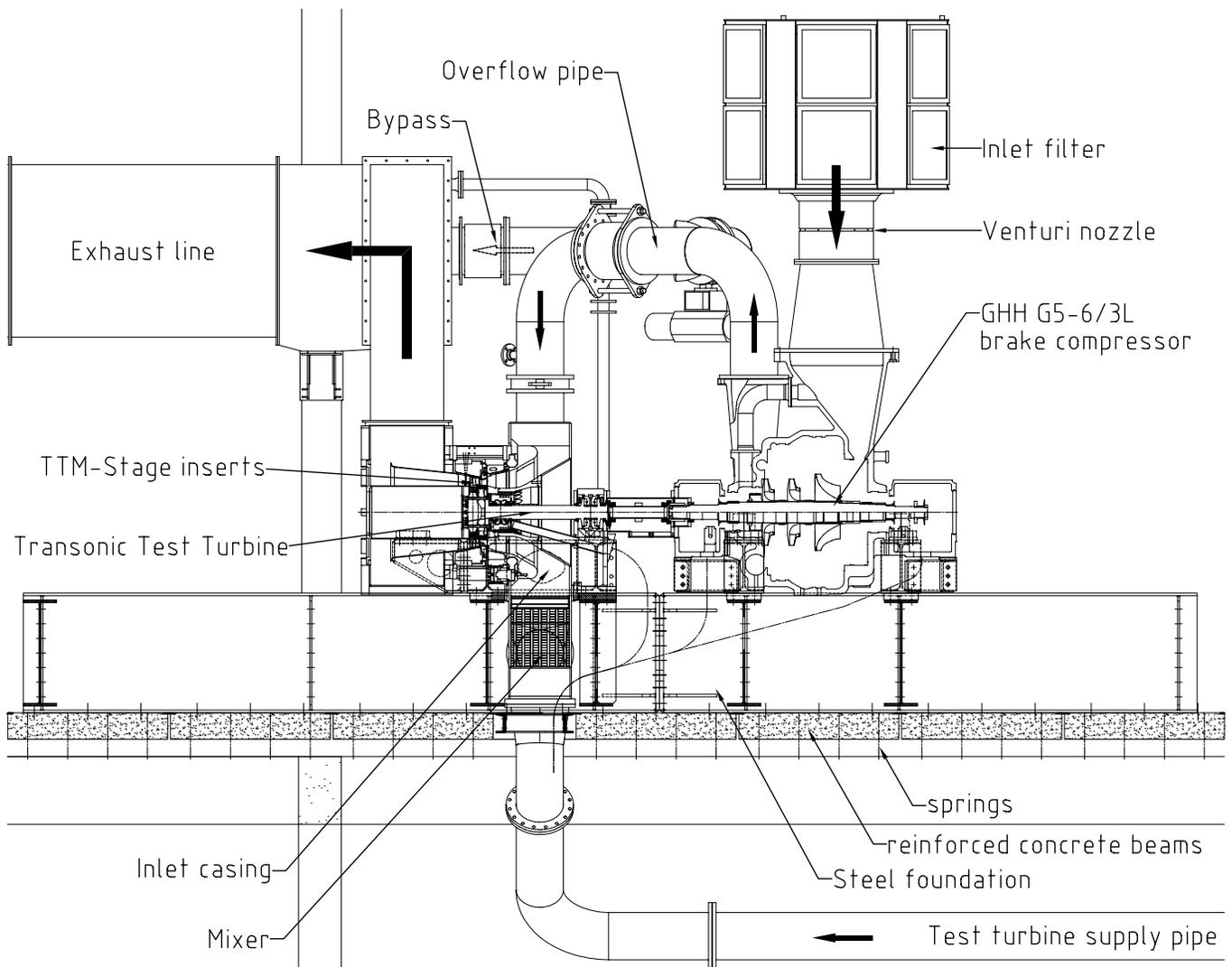
Fig. 2 Transonic Test Turbine Facility section
