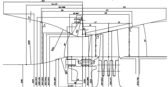
Fig. 8 Meridional Section TTM-Stage
