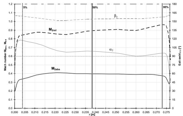
Fig. 13 Blade outlet conditions
