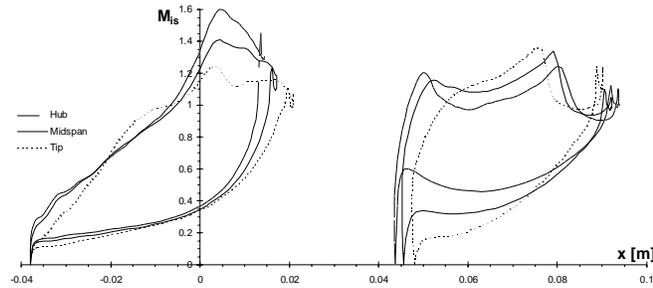
Fig. 10 Vane and blade surface Mach number distributions
