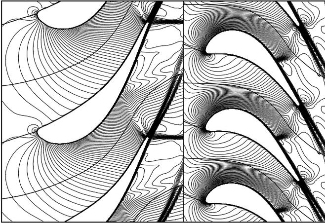
Fig. 6 Mach number contours at midspan predicted by viscous flow simulation (increment 0.02)
