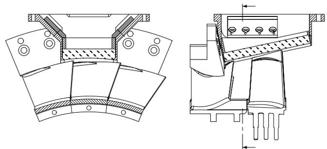
Fig. 4 Particle Image Velocimetry (PIV) window in TTM-Stage
