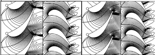
Fig. 7 Q3D-Euler predicted Pressure distribution (101, 0.5:4bar) nonreflecting boundaries left, reflecting outlet condition right
