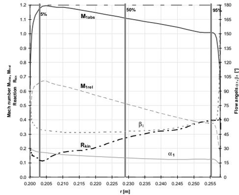
Fig. 12 Vane outlet / Blade inlet conditions
