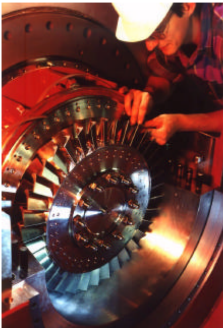
Figure 6: View of turbine rotor
