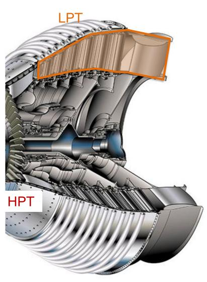
The Low Pressure Turbine (LPT) plays an important role in increasing the efficiency of an aero engine.
