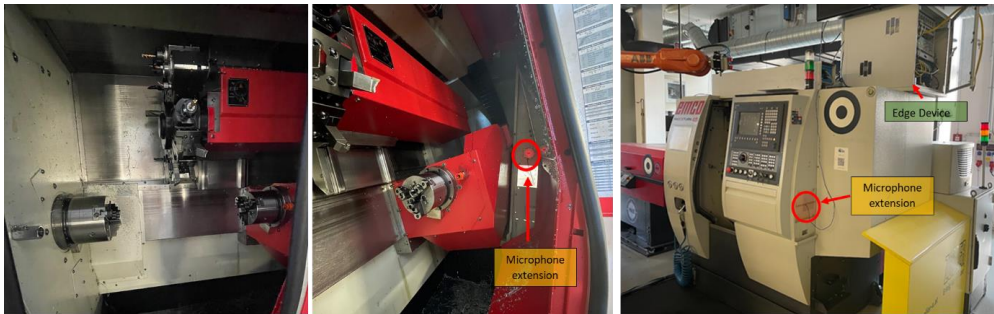
Maxxturn45 CNC machine with the position of the sensor and edge device
