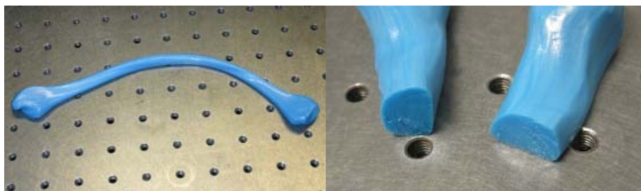
When stretched slowly, the Silly Putty flows while it breaks like a solid if pulled too quickly.
